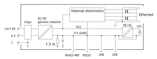
The operator panel has galvanic isolation against the 24 V DC feed but no galvanic isolation between the communication ports for RS232, RS422/485 and USB. Only the Ethernet connection has galvanic isolation.
