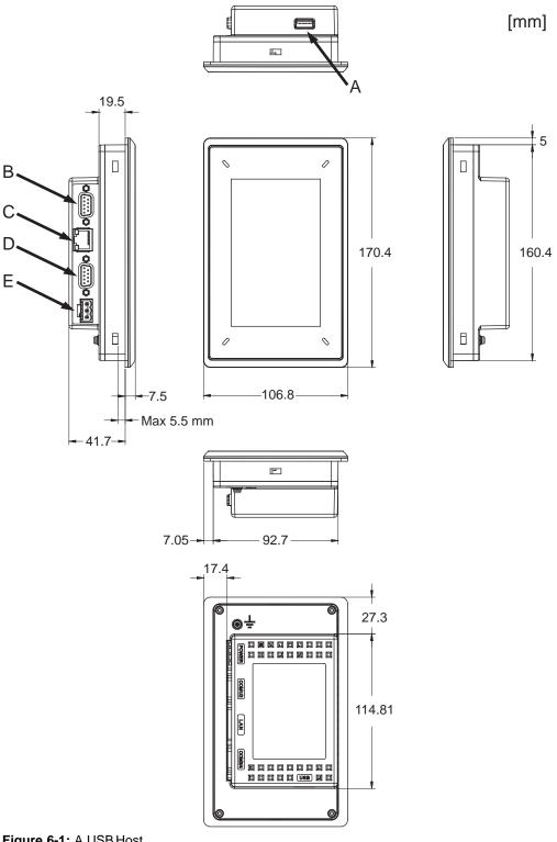
Figure 6-1: A.USB Host Figure 6-2: B. COM3/COM4 Figure 6-3: C. Ethernet Figure 6-4: D. COM1/COM2 Figure 6-5: E.24V DC
