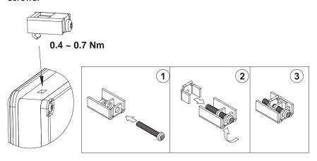
5. Connect the cables in the specified order, according to the drawing and steps below.
