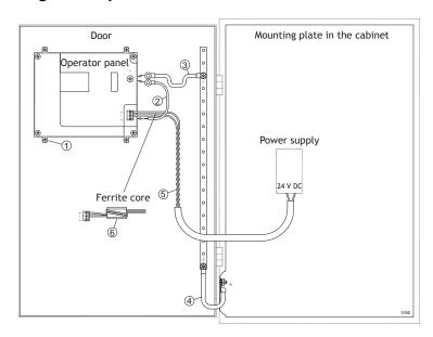
The mounting clamps of the HMI panel do not provide a secure grounding connection between the panel and the device cabinet, see 1 in drawing above.
