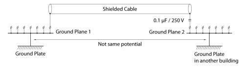
With longer distances, there is a risk that the ground potential may be different. In this scenario, the shield should only be connected at one end. A preferred alternative is to connect the other end of the shield to the ground via a 0.1 uF/250 V plastic capacitor. Both ends are then connected to the ground in terms of HF, but only connected to the ground at one end in terms of LF, thus avoiding the 50 Hz grounding loops.
