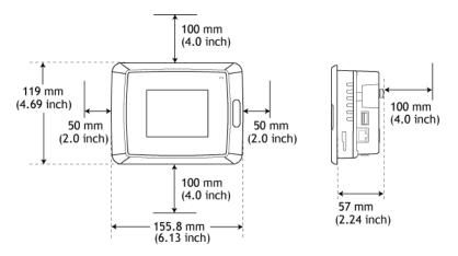
**CAUTION!** The openings on the enclosure are for air convection. Do not cover these openings!
