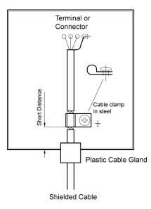
Use an EMC cable gland or regular plastic cable gland. Remove the outer jacket and connect the shield to the installation plate with a 360 ° metal cable clamp.
