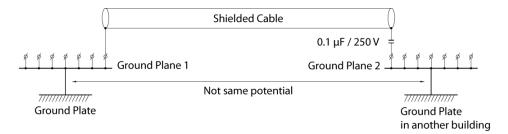
With longer distances, there is a risk that the ground potential may be different. In this scenario, the shield should only be connected at one end. A preferred alternative is to connect the other end of the shield to the ground via a 0.1 uF/250 V plastic capacitor. Both ends are then connected to the ground in terms of HF, but only connected to the ground at one end in terms of LF, thus avoiding the 50 Hz grounding loops.
