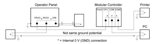
When a PC is connected to the terminal, the terminal's internal 0 V (GND) is connected to the protective ground via the PC.
