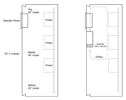
In most cases, the ambient temperature for the graphic operator terminal is significantly higher than the device cabinet's ambient temperature.
