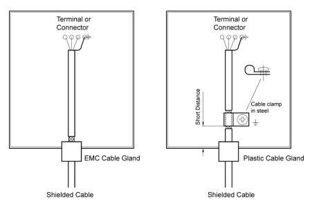
Use an EMC cable gland or regular plastic cable gland. Remove the outer jacket and connect the shield to the installation plate with a 360 ° metal cable clamp.
