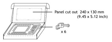
**WARNING!** Place the graphic operator terminal on a stable surface during installation. Dropping it or letting the terminal fall may cause damage.
