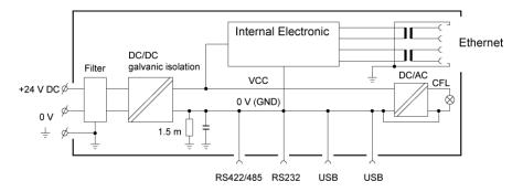
The graphic operator terminal has galvanic isolation against the 24 V DC feed but no galvanic isolation between the communication ports for RS232, RS422/485 and USB. Only the Ethernet connection isolation has galvanic isolation.
