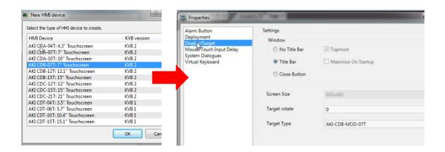
Additionally, the PxMM's IP address is also transferred into the KVB project when it is opened from within the KAS IDE.
