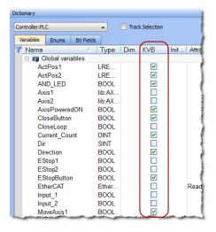
The Modbus tag addresses are defined automatically in the KAS IDE when the project is compiled, then transferred into KVB when the KVB project is opened from inside the IDE. Global or local variables can now be selected to share over Modbus. Each time the KAS IDE project is compiled the share list is updated.
