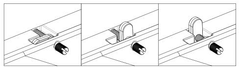
Figure 3-1: Tighten the screws to  $0.7 \, \text{Nm} \pm 0.2 \, \text{Nm}$ .
