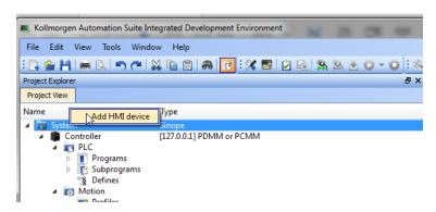
This selection is transferred into KVB when it is opened from inside the KAS IDE.
