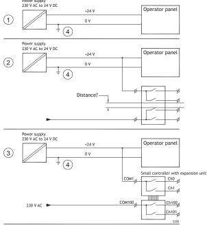
If a power supply that meets safety standards is used and only feeds the operator panel, there is no problem. See 1 in drawing above.
