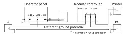
When a PC is connected to the HMI panel, the internal 0 V (GND) of the panel is connected to the protective ground via the PC.
