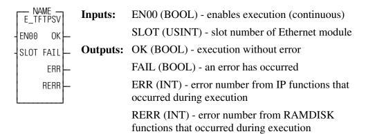
This function block allows a PiC or MMC to service TFTP file transfer requests for a file on the RAMDISK.
