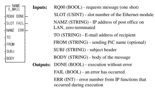
This function block enables a PiC or MMC to send a text-based e-mail message via SMTP using the Ethernet module. This function block does not allow the PiC or MMC to receive or respond to e-mail.
