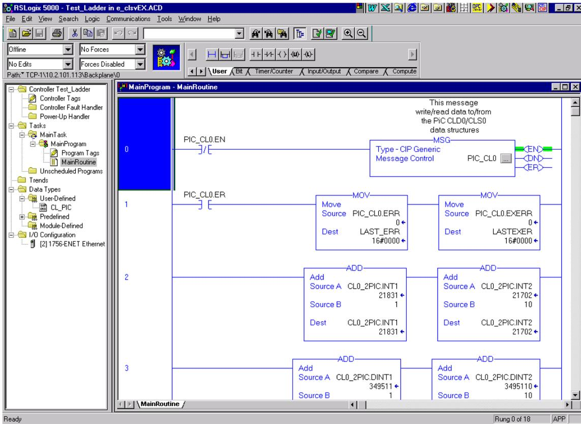
2. Access the Message Configuration window by double clicking on the MSG function. Fill in the data fields for the Configuration tab as follows.
