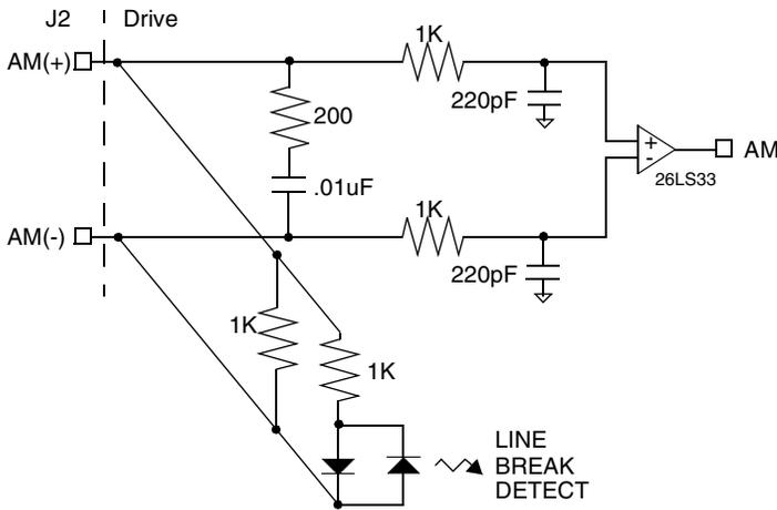
FIGURE 6.35 Motor Encoder Interface Circuit
