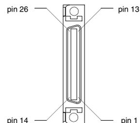
J3 is a 26 pin female mini-D ribbon connector (AMP 2-178238-4). It duplicates the first 26 pins of J1, the Controller connector, which are discussed in detail beginning on page 6-53. Contact between the connector shell and the grounded chassis provides shield termination.
