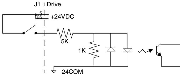
**FIGURE 6.2 Drive Input Connected to a Switch/Relay Contact**
