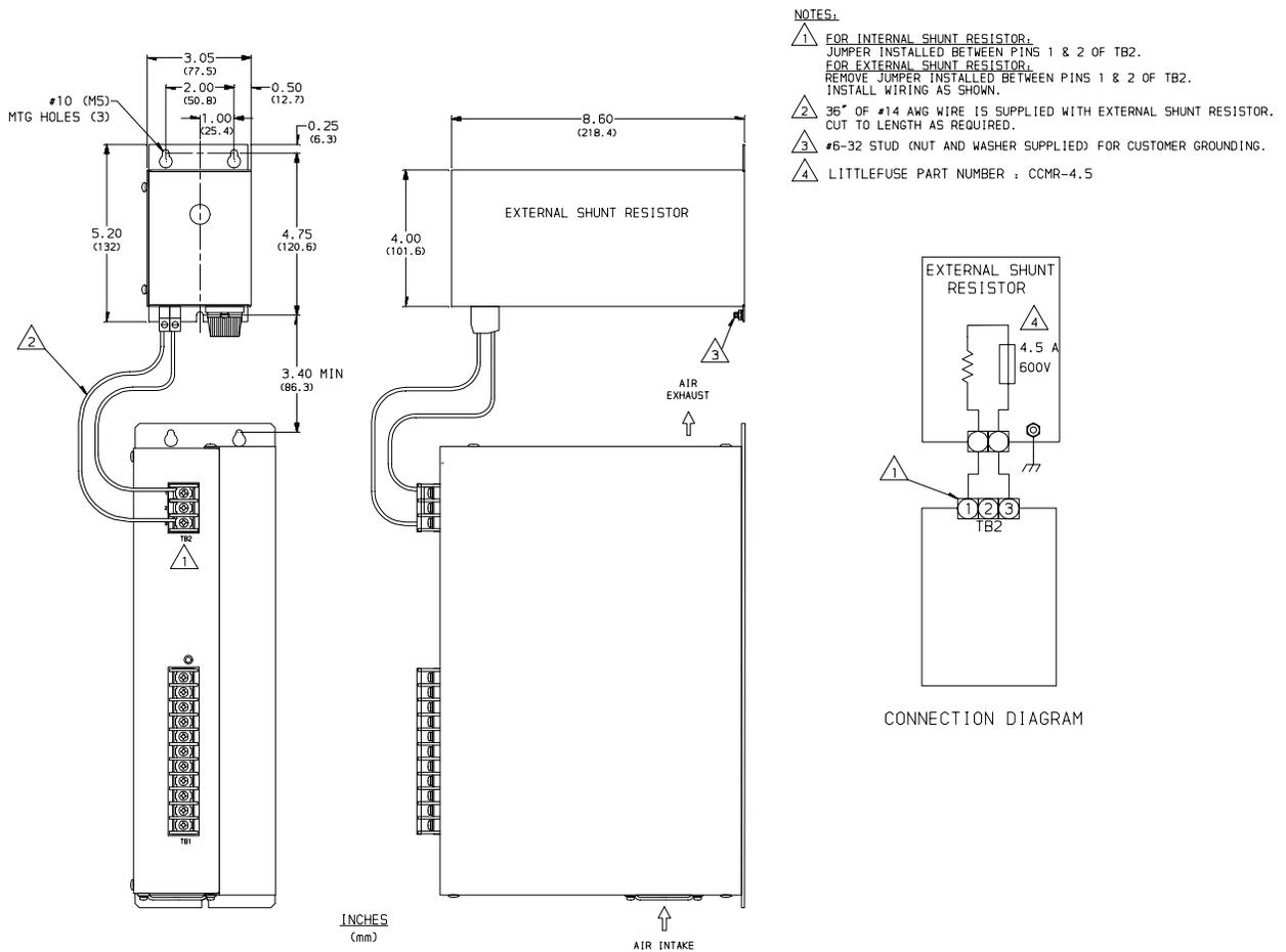
FIGURE 7.5 External Shunt Mounting Diagram
