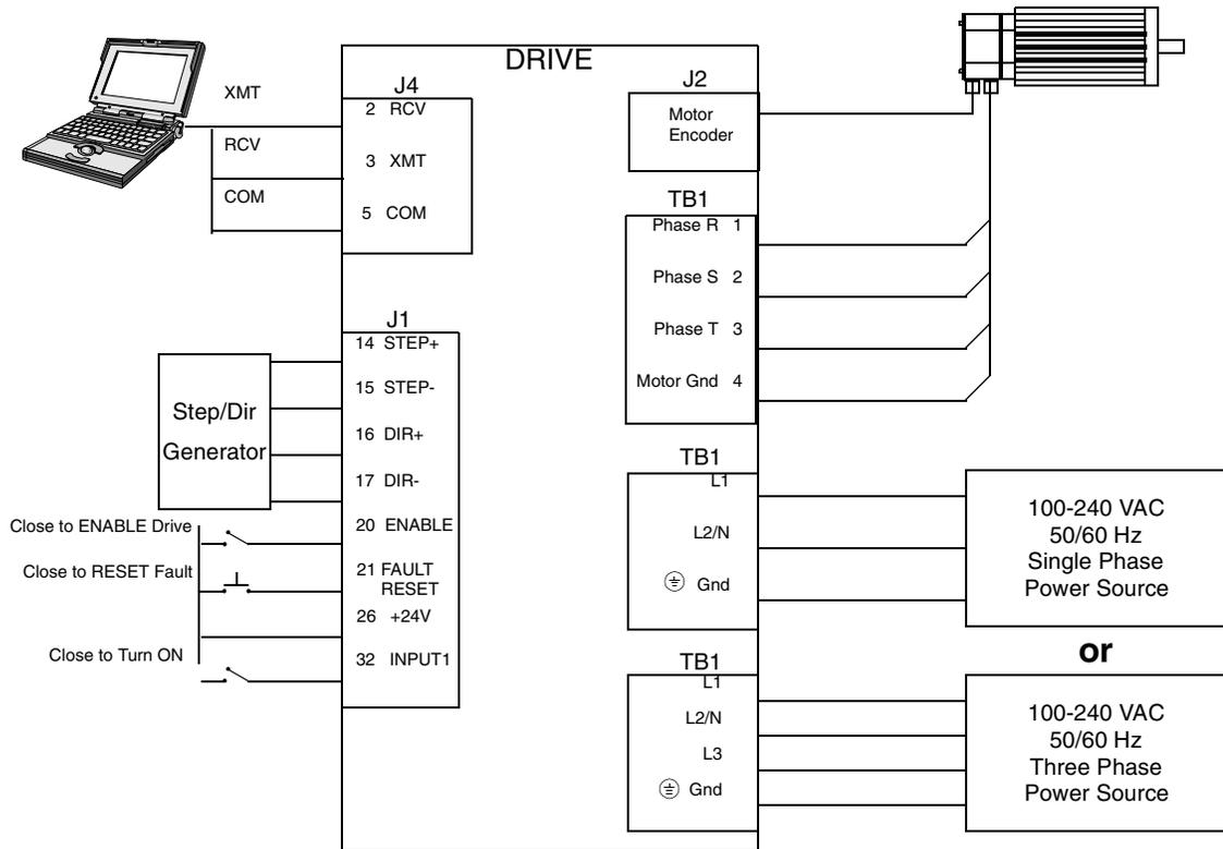
Note 1. Refer to Figure 6.31 and 6.32 for additional details on the Control Interface Cable.
