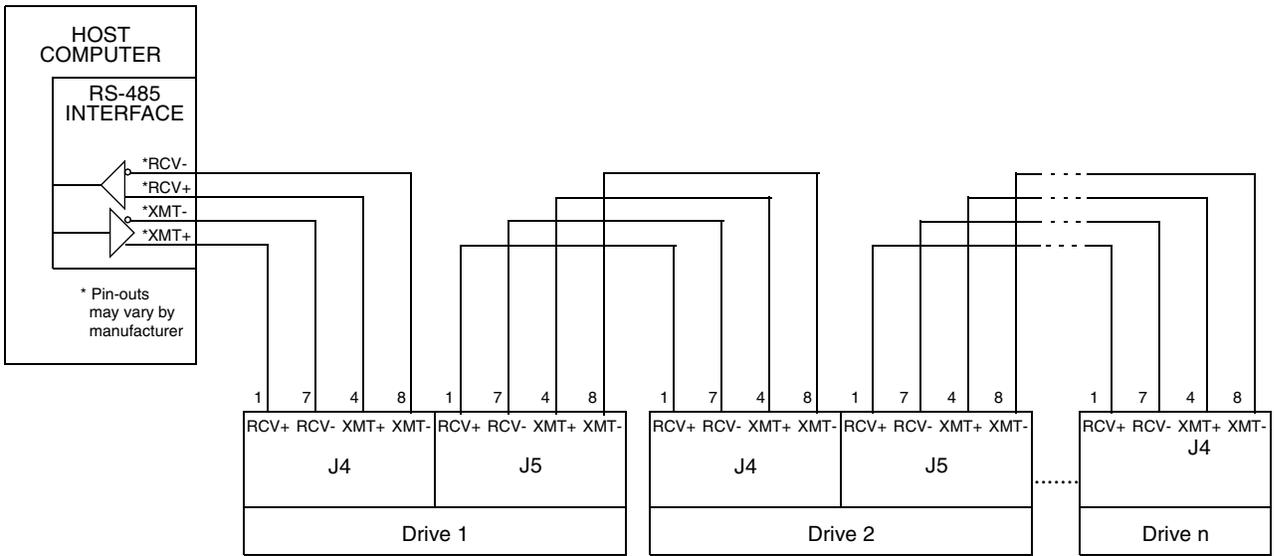
FIGURE 6.42 Four Wire RS-485 Daisy Chain Connection Diagram
