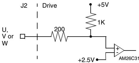
FIGURE 6.36 Hall Effect Sensor Circuit
