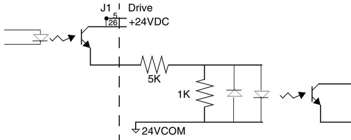
**FIGURE 6.3 Drive Input Connected to an Opto-Isolator**
