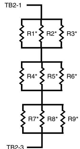
NOTES: A single resistor of equivalent total resistance may replace multiple resistors.
