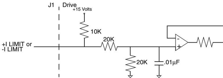
FIGURE 6.17 Positive and Negative Current Limit Circuits
