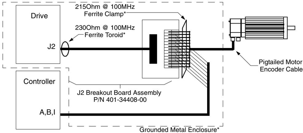
NOTE: An asterisk (\*) indicates an installation option to comply with EU EMC Directives. Either a grounded metal enclosure or ferrite cores provide the requisite EMC protection.
