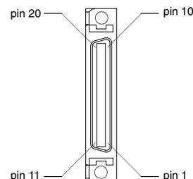
J2 is a 20 pin female mini-D ribbon connector (AMP 2-178238-2). It connects the motor encoder, hall effect switches, and the thermostat to the Centurion DSM100 Drive. Contact between the connector shell and a grounded chassis provides shield termination.
