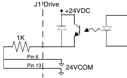
FIGURE 6.12 Drive Output Connected to a Resistive Load
