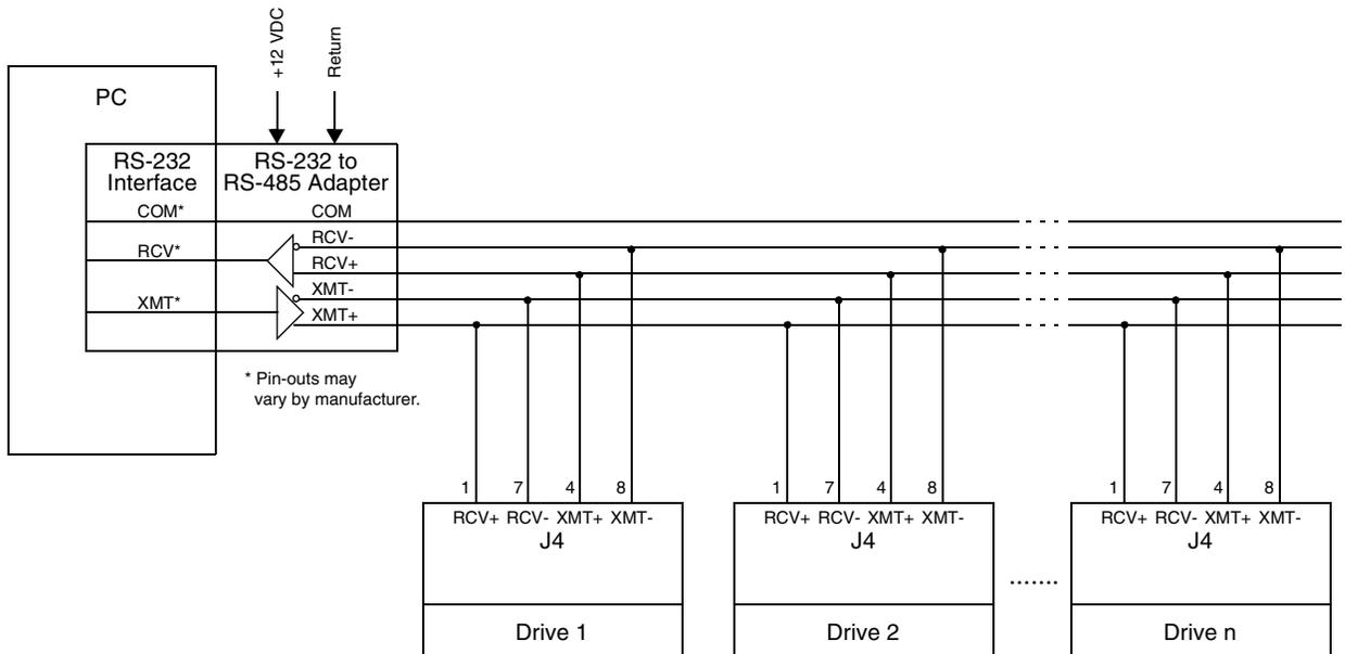
FIGURE 6.43 RS-232 to RS-485 Multi-Drop Connection Diagram
