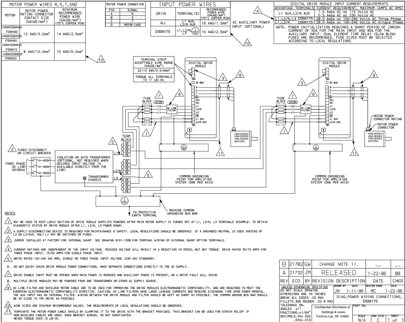
FIGURE 5.5 Power Wiring Diagram for DSM175 and DSM175P
