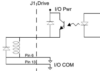
FIGURE 6.13 Drive Output Connected to a Switch/Relay
