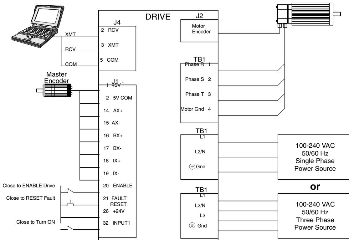
Note 1. Refer to Figure 6.24, 6.25, 6.26, 6.27, 6.28, 6.29 and 6.30 for additional details on the Control Interface Cable.
