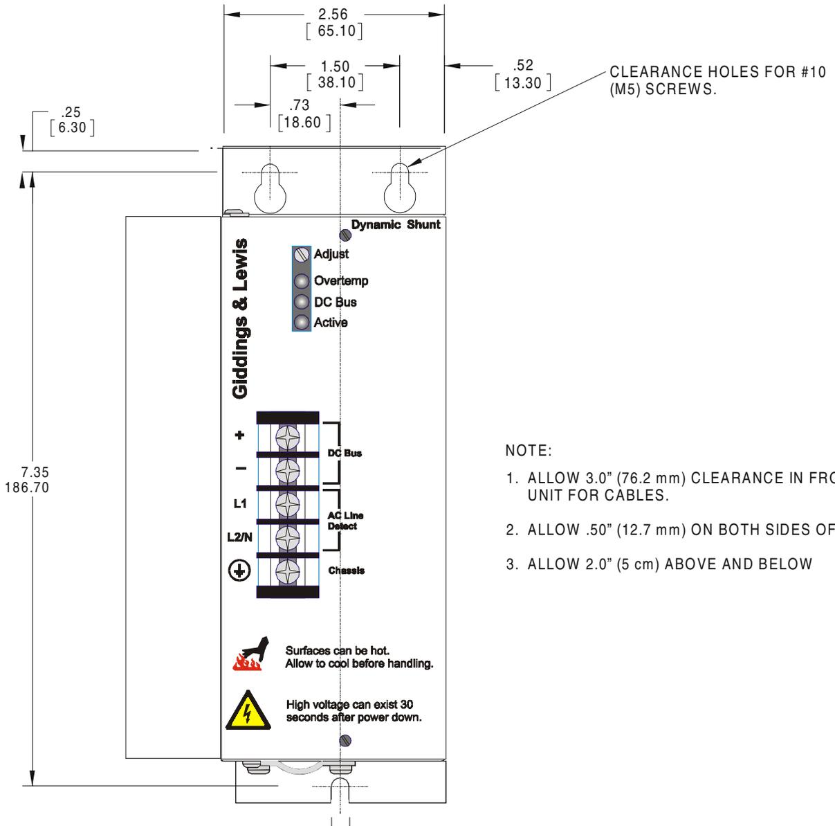
CLEARANCE HOLES FOR #10 (M5) SCREWS.
