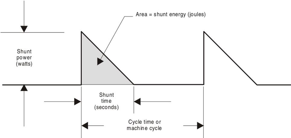
Shunt power is the peak shunt power during the shunt time. Shunt time is the time the power pulse is dissipated by the shunt. The cycle time is the time from the beginning of one shunt to the beginning of the next shunt time.
