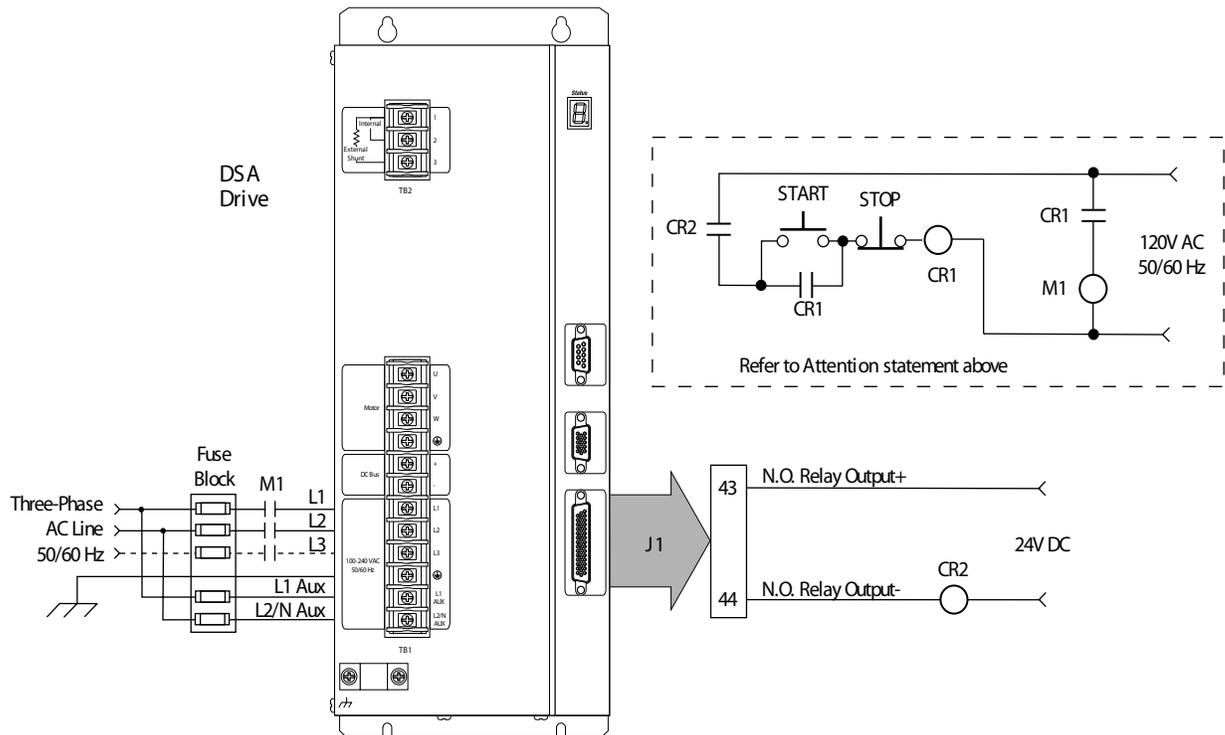
Note: Relay Output (pins 43 and 44) must be configured as Ready in DSA Drive software.
