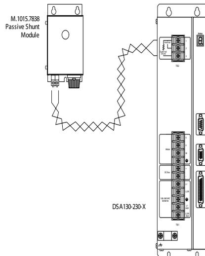
Use shielded, high temperature 75° C (167° F), 600V, 2.5 mm<sup>2</sup> (14 AWG), 3.05 m (10 ft) maximum, copper wire. Follow one of the methods given below to reduce the effects of EMI noise:
