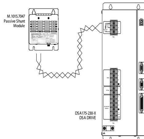
Use shielded, high temperature 75° C (167° F), 600V, 10 mm<sup>2</sup> (8 AWG), 3.05 m (10 ft) maximum, copper wire. Follow one of the methods given below to reduce the effects of EMI noise:
