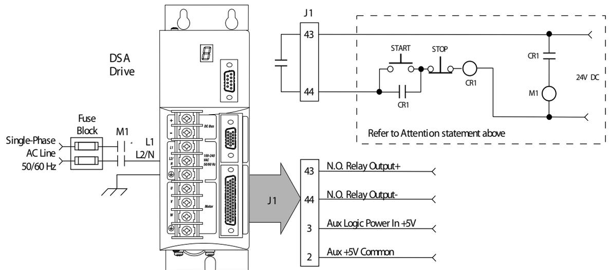
Note: Relay Output (J1, pins 43 and 44) must be configured as Ready in DSA Drive software and auxiliary +5V power is required.
