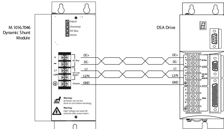
Use shielded, high temperature 75° C (167° F), 600V, 2.5-4.0 mm<sup>2</sup> (12-14 AWG), 3.05 m (10 ft) maximum, copper wire. Follow one of the methods given below to reduce the effects of EMI noise:
