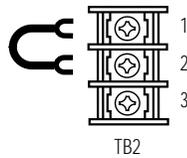
Connecting the External Shunt Resistor
