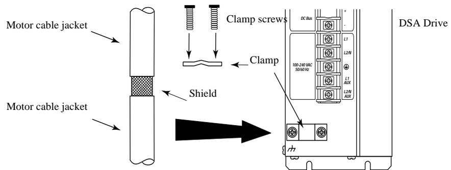
YSM Series motors have a short pigtail cable which connects to the motor, but is not shielded. These motor power cables have a 152.4 mm (6.0 in.) shield termination wire with a ring lug that connects to the closest earth ground. The termination wire may be extended to the full length of the motor pigtail if necessary, but it is best to connect the supplied wire directly to ground without lengthening. Refer to Figure 3.6 for an illustration.
