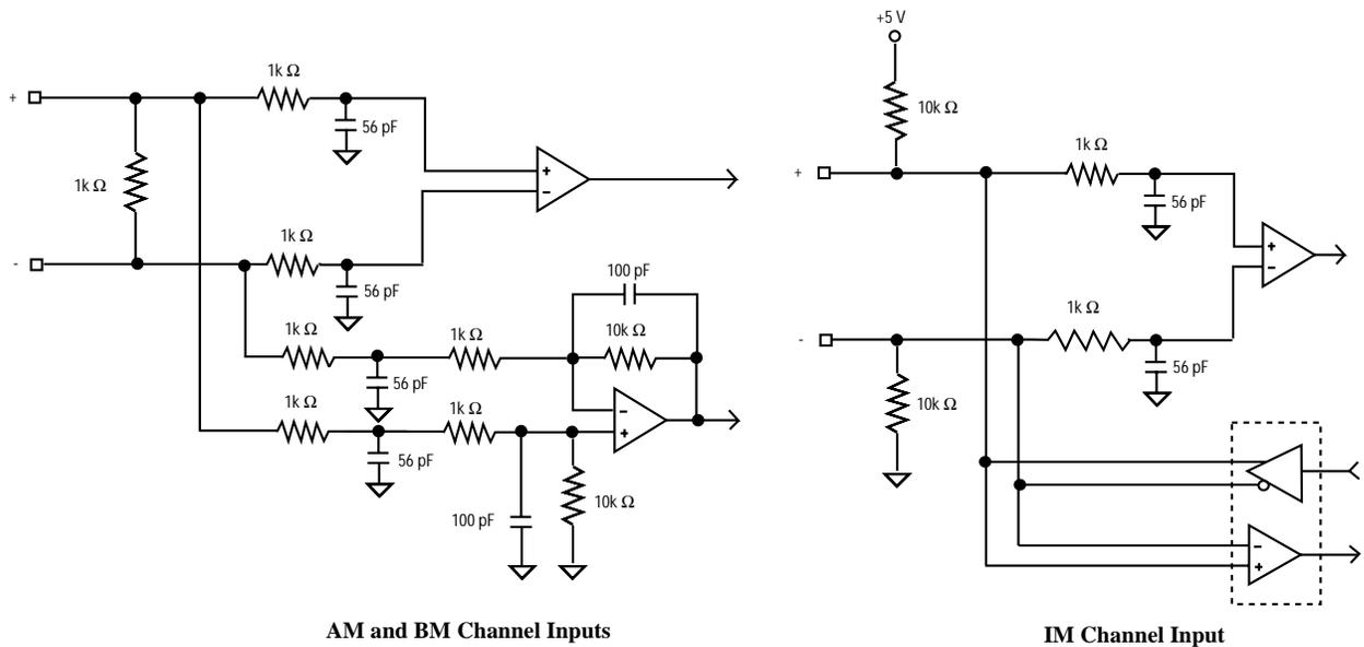
The DSA Drive supports both TTL and Sine/Cosine encoders. The following table provides a description of the AM, BM, and IM inputs for TTL encoders.
