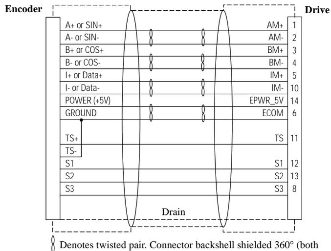
**IMPOR-** Total resistance of the wiring for encoder power and ground connections between the drive and motor must be less than 1.4 ohms.
