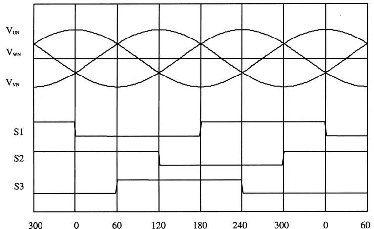
Figure 2.23 shows the proper phasing of TTL A/B encoder signals when positive current is applied.
