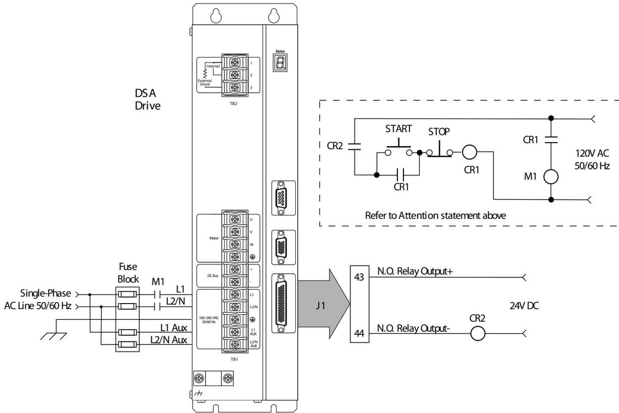
Note: Relay Output (pins 43 and 44) must be configured as Ready in DSA Drive software.
