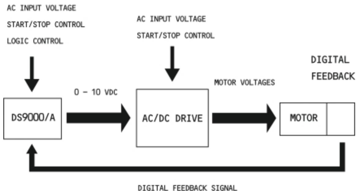
Figure 1 Standard DS9000/A Connection Requirements
