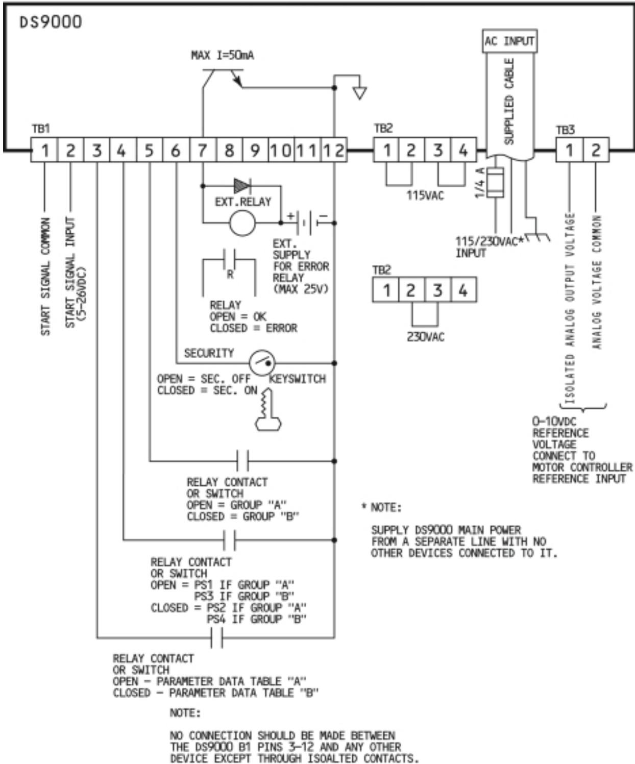
Figure 1 – Connection Diagram
