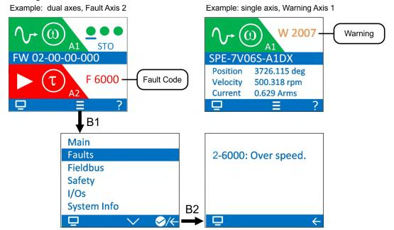
You can retrieve faults on a per-axis basis with the keyword: AXIS#.FAULTS, where # is the Axis number.
