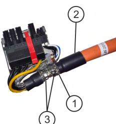
Strip the external cable sheath to a length of approx. 80 mm, taking care not to damage the braided shield. Push the braided shield (1) back over the cable and secure with a rubber sleeve (2) or shrink sleeve.
