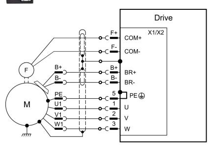
Pinout is identical for connectors X1 and X2.
