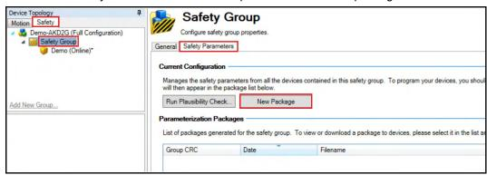
The safety parameters are bundled to a package in the "Parameterization Packages" screen
