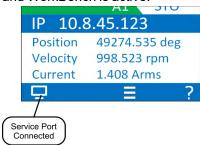
Use WorkBench to configure the drive by using the service interface.
