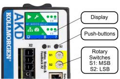
The display on the front panel of the drive shows the code of the fault or warning that occurred. Safety Faults and Warnings follow the same pattern and are identified by a four digit code 90 XX, where 90 is the two digit group code, and XX is a two digit ID.
