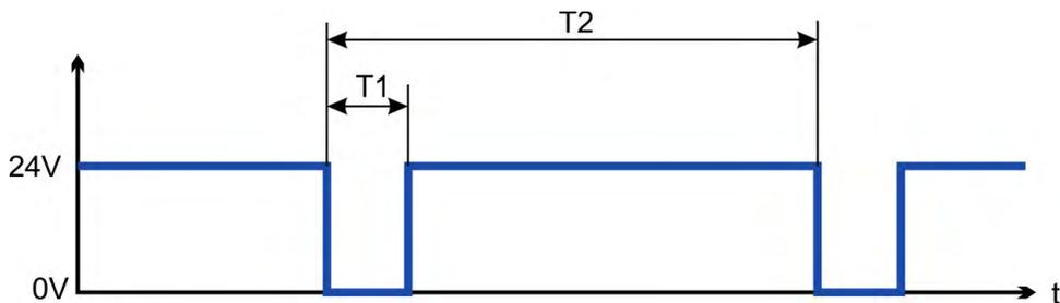
Test pulses with  $T1 < 300 \mu s$  and  $T2 > 200 ms$  will not have any influence to the safety relevant STO function. Test pulses, which are outside of this specification, will switch the STO function, but will not create a dangerous situation.
