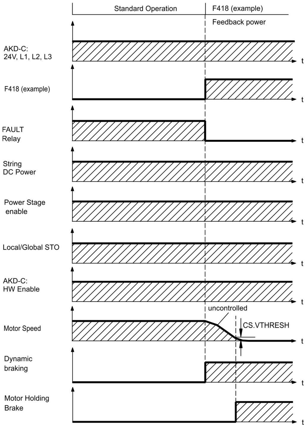
If velocity drops below threshold  $CS.VTHRESH$  or timeout occurs brake is applied .
