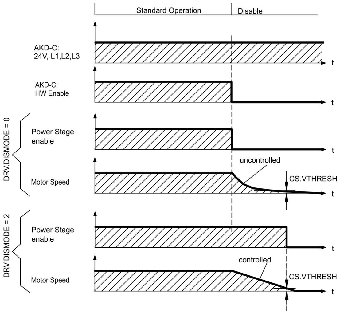
If velocity drops below threshold  $CS.VTHRESH$  or timeout occurs the motor holding brake is applied. Set parameter `MOTOR.BRAKEIMM` to 1 with vertical axes, to apply the motor holding brake immediately after Hardware Disable.
