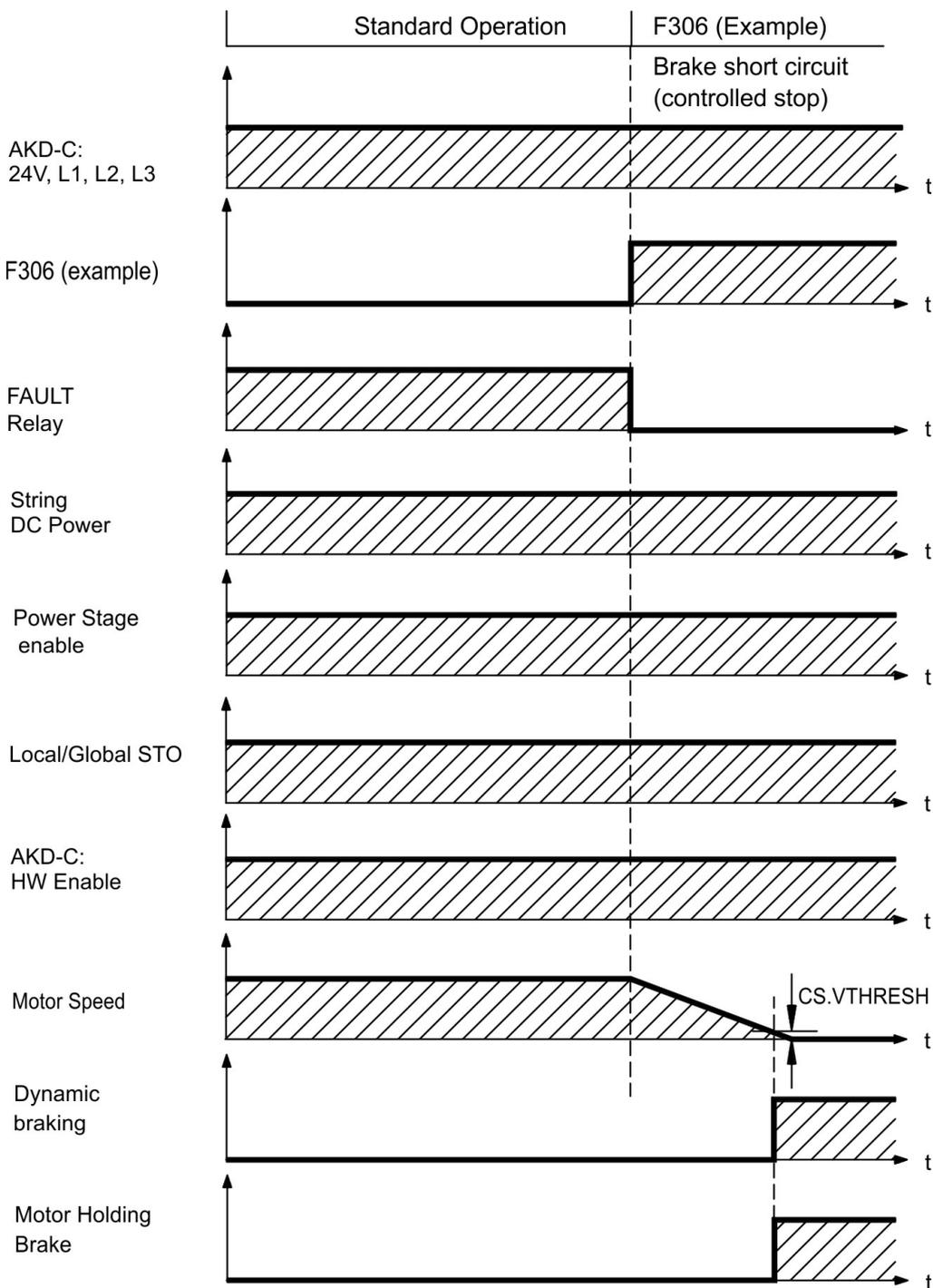
If velocity drops below threshold  $CS.VTHRESH$  or timeout occurs brake is applied .
