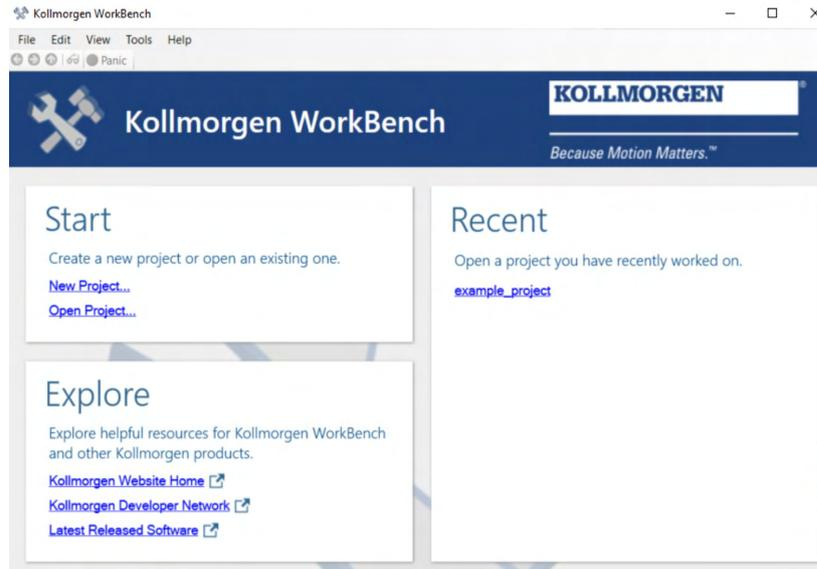
The setup software WorkBench for AKD-N and AKD-C devices is intended to be used for altering and saving the operating parameters for the decentral drive system. The attached device can be set up with the help of this software, and during this procedure the drive can be controlled directly by the service functions.
