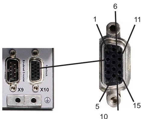
**Figure 7. Feedback Connection**
