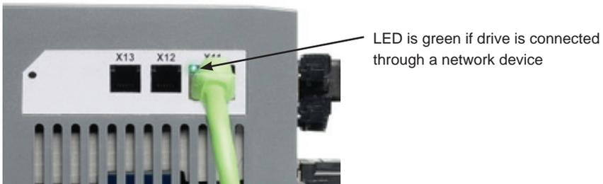
**Figure 15. Active connection LED**
