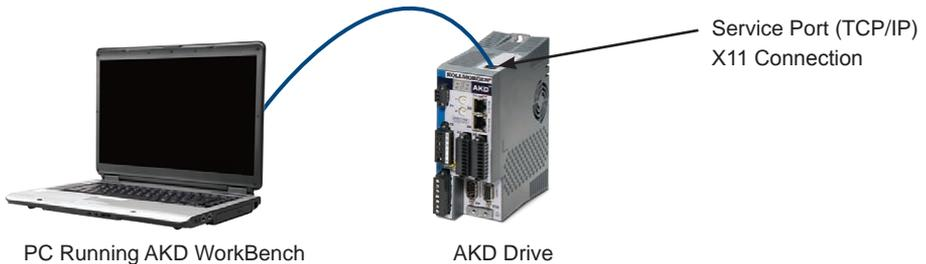
**Figure 12. Option A: Direct Connection**
