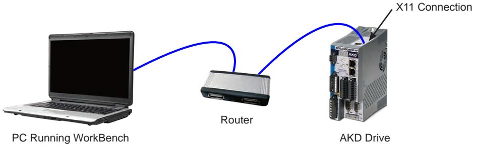
**Figure 14. Option B: Connection to a Router**
