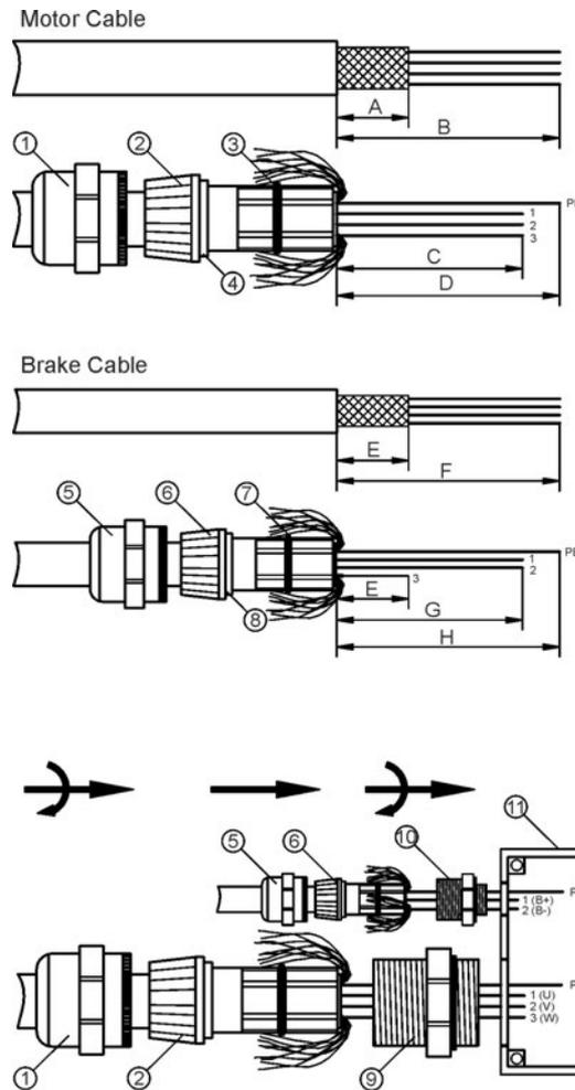
Remove the outer covering over length B, without damaging the shielding braid. Shorten the shielding braid to length A.
