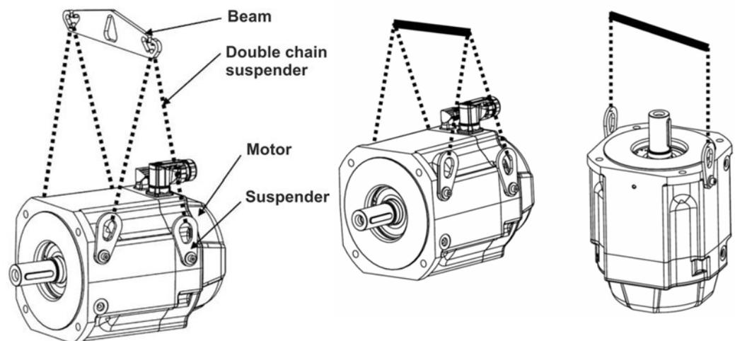
The suspended unit consists of a Beam, suspended off the crane hook and two double-run chain suspenders. The motor may be borne on two or four runs of the chain suspender.
