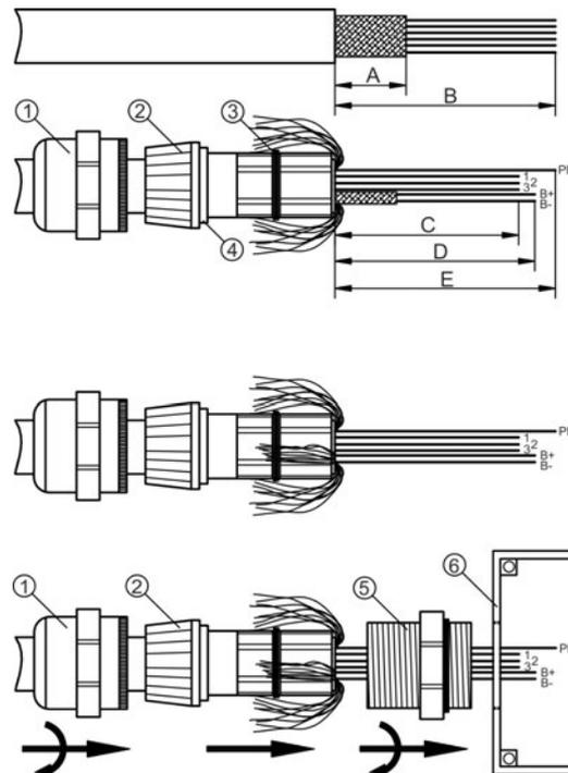
Remove the outer covering over length B, without damaging the shielding braid. Shorten the shielding braid to length A.
