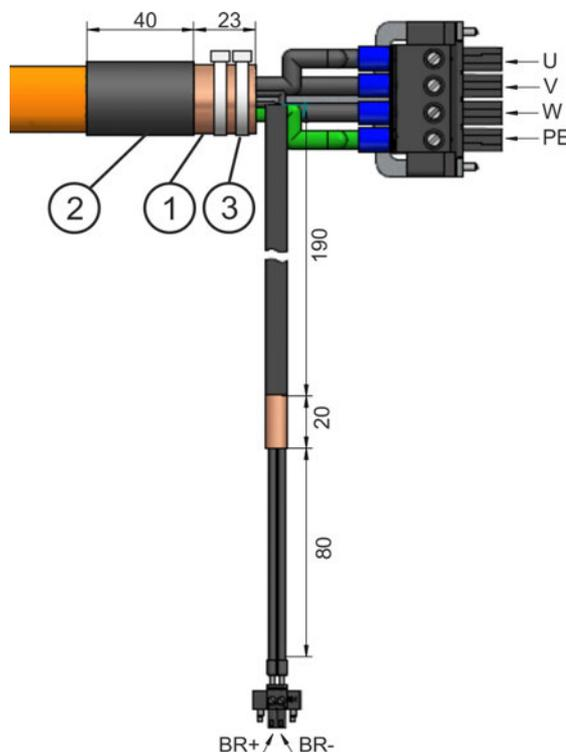
Strip the external cable sheath to a length of approx. 300 mm, taking care not to damage the braided shield. Push the braided shield (1) back over the cable and secure with a rubber sleeve (2) or shrink sleeve.
