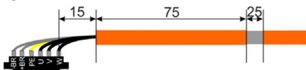
The motor is connected to the AKD-x00306/x00606 with a connector (→ p. 56). Please take note that the connector can accept a maximum conductor cross-section of 4 mm<sup>2</sup>.
