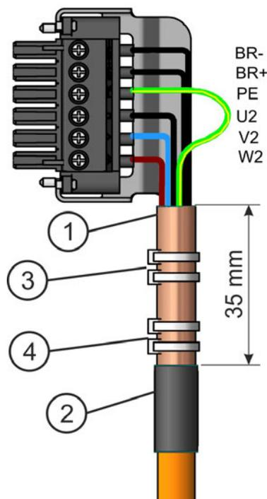
Strip the external cable sheath to a length of approx. 120 mm, taking care not to damage the braided shield. Push the braided shield (1) back over the cable and secure with a rubber sleeve (2) or shrink sleeve.
