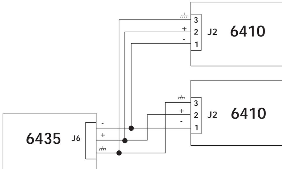
**Note:** If the 6435 is powering additional 6410s with J6, a total of 1000  $\mu\text{f}$  (maximum) 100 Vdc aluminum electrolytic capacitor, rated for 2A ripple current or greater @ 10 KHz and 105°C, must be installed at the 6410 (as close to the 6410 as possible) if the cable length is over 3 feet. **DO NOT** exceed 1000  $\mu\text{f}$  total on J6 external connector.
