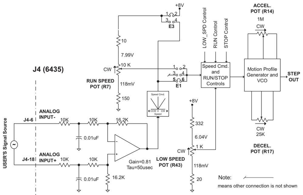
**External analog input with internal RUN SPEED pot**
