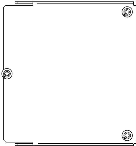
4. Fasten cover to hex standoffs using two of the screws provided.
