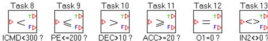
Comparison blocks compare a parameter to a value and flow continues according to the comparison. There is a single input flow path and two output flow paths, True (T) and False (F).
