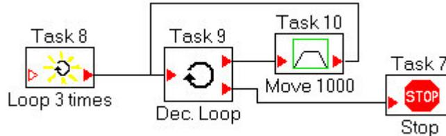
*A Decrement Loop Block is normally placed immediately after an Initialize Loop Block*
