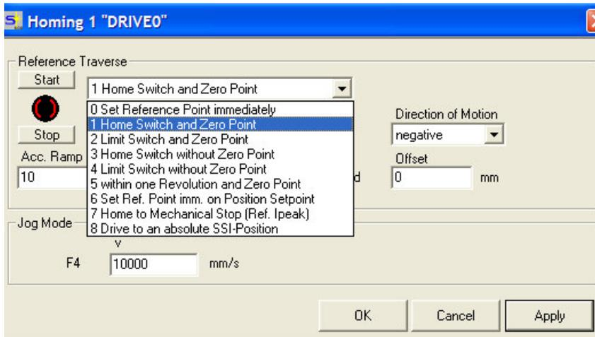
Other homing types that have movement require additional setup on this screen: Velocity, Acceleration, Deceleration, Move Direction, and Home Position Offset. IF the home type requires a home switch and/or limit switch, the digital inputs on connector X3 must be configured for this functionality. If the OPT-IO option card is used the home input is also available on this connector.
