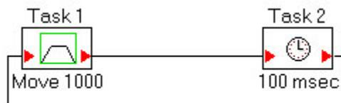
When the download to drive button is clicked on in GMT the program is first converted into ORDER commands, displayed in the Motion Task Table, and loaded into the S600 memory. Each block in GMT is converted into one ORDER command. The S600 can store 255 ORDER
