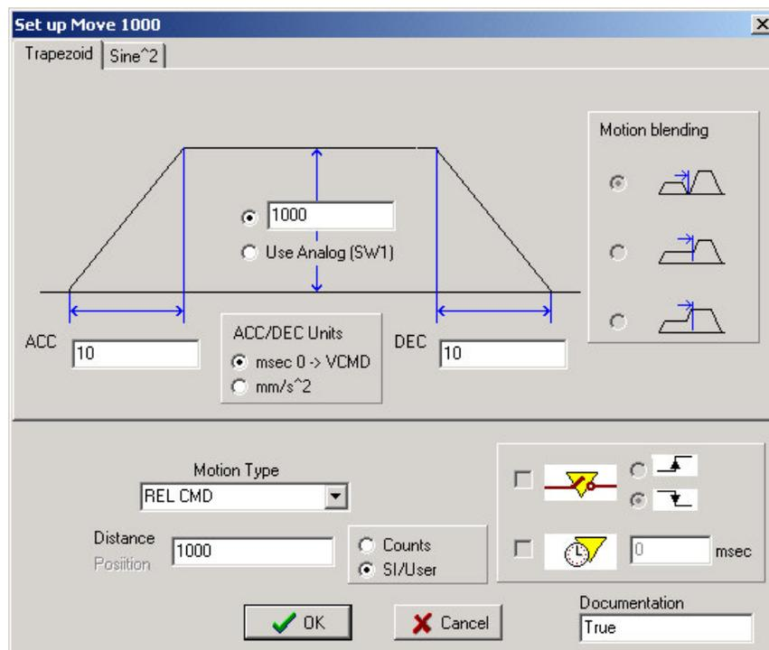
Using this screen, you can set acceleration and velocity variables in the top left area. The motion type (Relative, Absolute, etc.) and the target position/distance are set at the bottom left of the screen. Normally, you select SI/User units. “Counts” are internal units. Consult product documentation for more information on SERVOSTAR S600 units.
