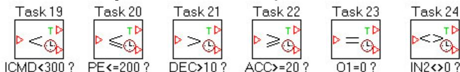
Timed comparison blocks compare a parameter to a value and flow continues according to the comparison. There is a single input flow path and two output flow paths, True (T) and False (F). Flow continues through the false path only after the false condition is present for the timeout period.
