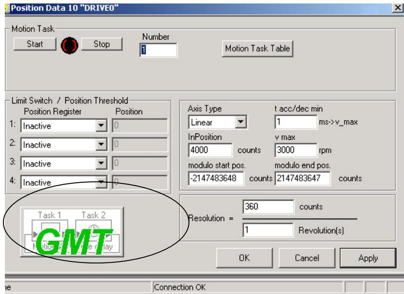
The Graphical Motion Tasking programming environment shown below has several controls at the top left, motion tasking blocks at the top right, and the GMT canvas at the bottom. The figure below includes a simple GMT program that indefinitely repeats a 1000-count move followed by a 100 msec time delay.
