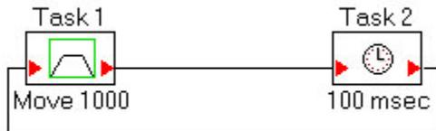
This program is stored in the Drive.exe Motion Task Table. It can be viewed by going to the Position Data Screen and clicking on “Motion Task table”:
