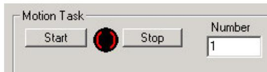
Specify the starting task order number using the edit box marked *Number* to the right of the Motion Task *Stop* button. The order number is shown above each block that represents a motion task.
