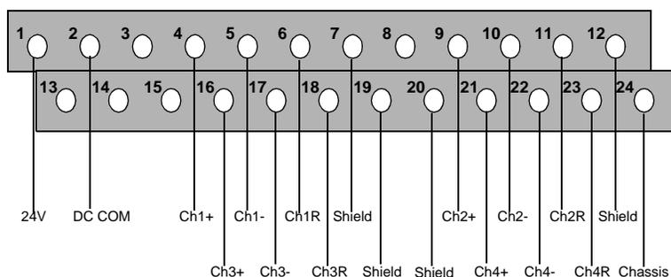
When connecting an analog voltage output device to the module, the positive wire of the twisted pair goes to the + screw terminal and the negative wire goes to the - screw terminal. Figure 11-3 illustrates these connections for channel one.
