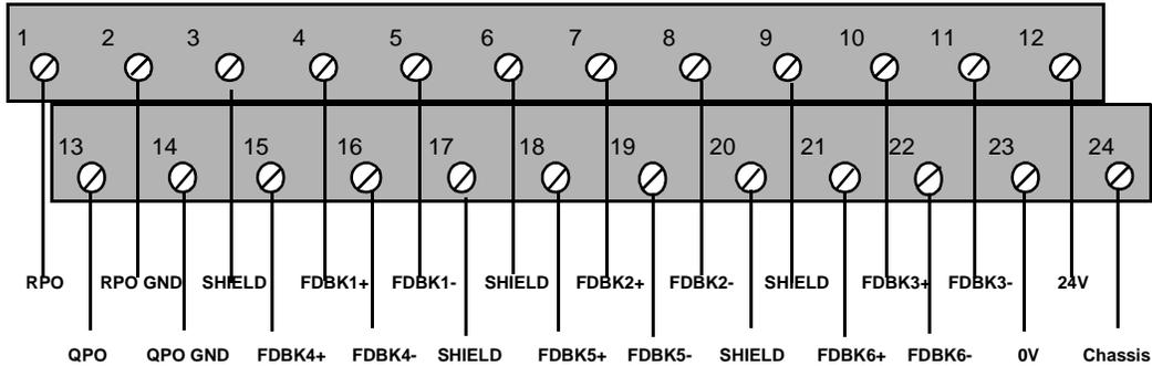
To connect six resolvers to the block resolver module, a user-supplied external terminal block must be used.
