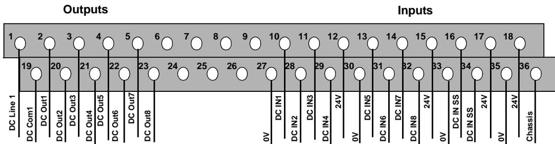
Typically, an external 24V DC supply is connected to pins 18 and 35. These pins are internally jumpered so that the supply is available at the other pins labeled as 24V and 0V. This makes it convenient to connect a 3-wire device (i.e., a proximity switch) which requires a voltage and ground connection. Also, 24V or 0V can be easily jumpered to the input sink/source connection.
