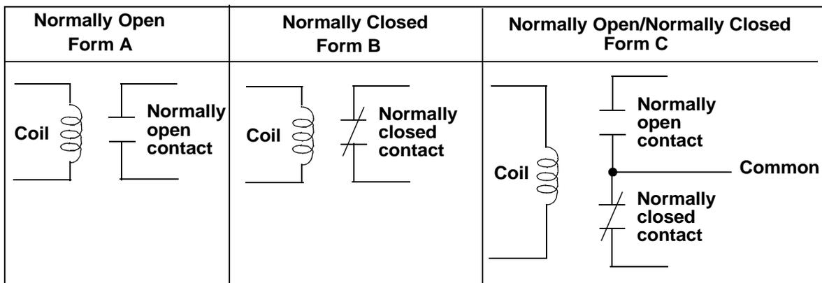
A relay is energized or de-energized according to the logic state sent to it by the CPU. If the CPU sends a logic 1, the relay is energized. If the CPU sends a logic 0, the relay is de-energized. The logic state for each relay is updated every time the CPU scans the ladder program.
