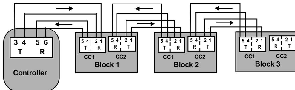
**NOTE:** CC represents the communication connections at the top of the block modules.
