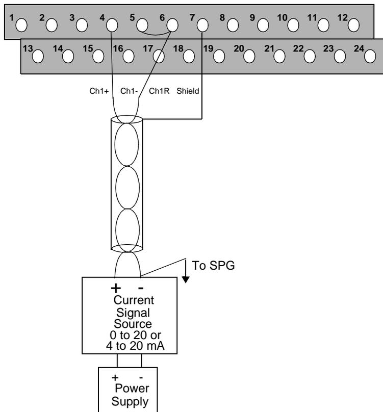
An alternative method of connecting a two wire 4 to 20 mA current device is shown in Figure 11-5. Place a jumper between the - input and the 250Ω resistor input.
