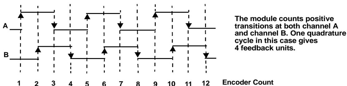
For each encoder channel, there is a 24-bit up/down counter. It is incremented or decremented in accordance with the signals received from the differential quadrature encoder. There is also a 24-bit latch associated with each encoder input channel.
