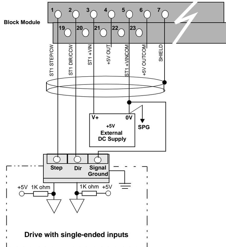
If the pull-up resistors internal to the drive are inadequate, you may need to add external pull-up resistors. Install them as close as possible to the drive.
