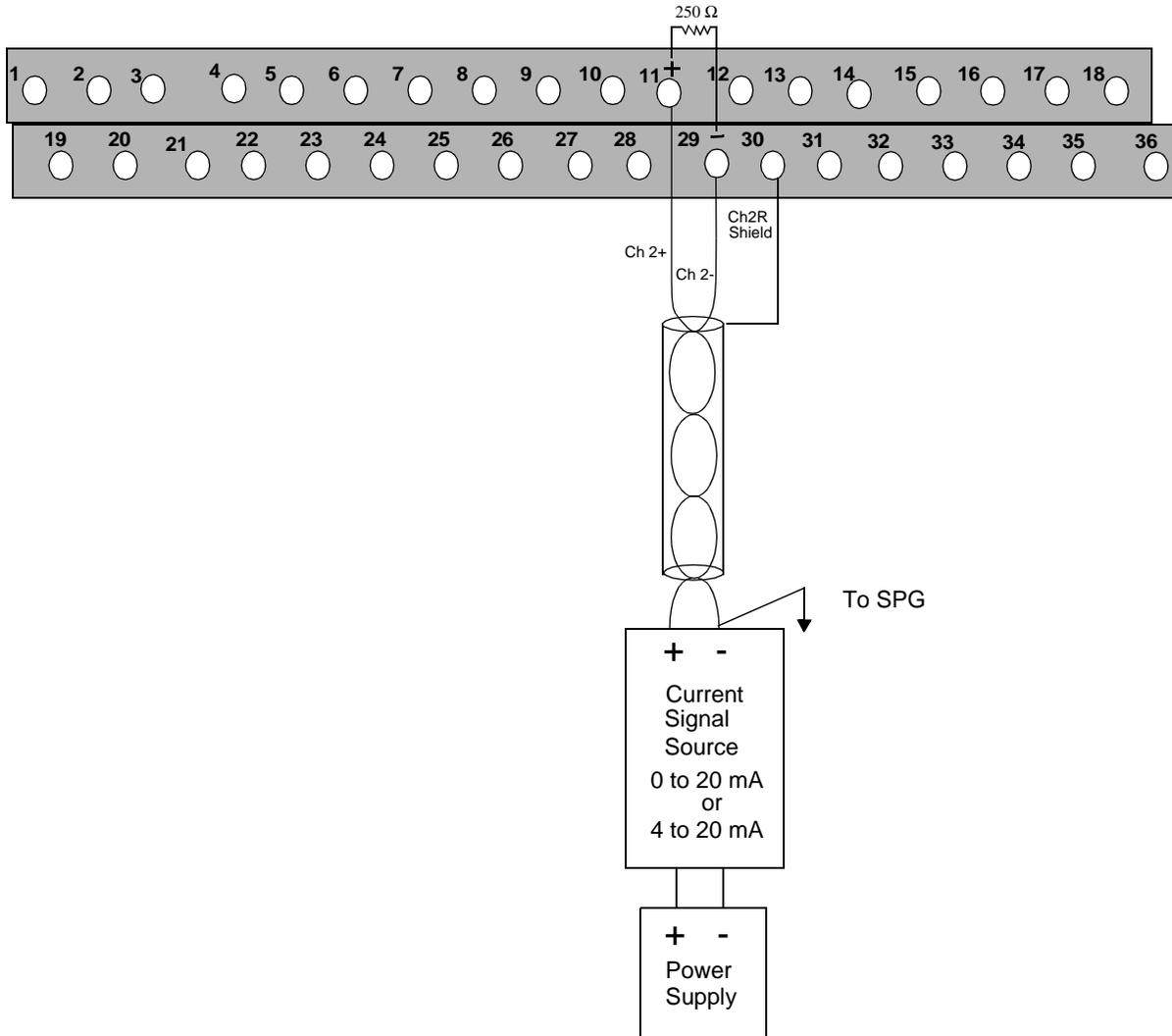
NOTE: The accuracy of the current input can be no more accurate than the accuracy of the 250  $\Omega$  resistor used.
