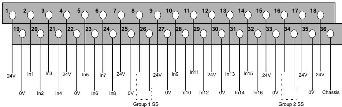
Typically, an external 24V DC supply is connected to pins 18 and 35. These pins are internally jumpered so that the supply is available at the other pins labeled as 24V and 0V. This makes it convenient to connect a 3-wire device (e.g., a proximity switch) which requires a voltage and ground connection. Also, 24V or 0V can be easily jumpered to a group's sink/source connection.
