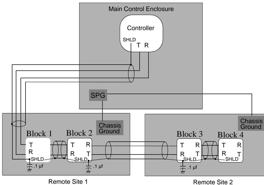
The distance between block I/O modules can be up to 200 feet.
