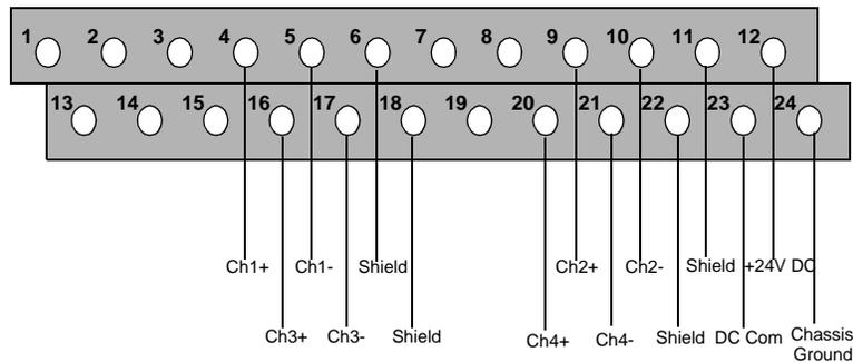
Each output channel is connected to a receiving device with twisted pair wires as shown in Figure 13-3. For extremely noisy environments, use shielded twisted pair wire.
