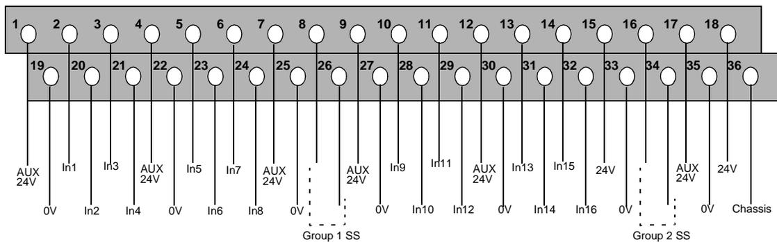
Typically, an external 24V DC supply is connected to pins 18 and 35.
