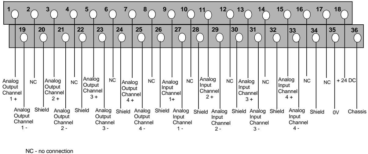
When connecting an analog voltage output device to the module, the positive wire of the twisted pair goes to the + screw terminal and the negative wire goes to the - screw terminal. Figure 16-3 illustrates these connections for channel two.
