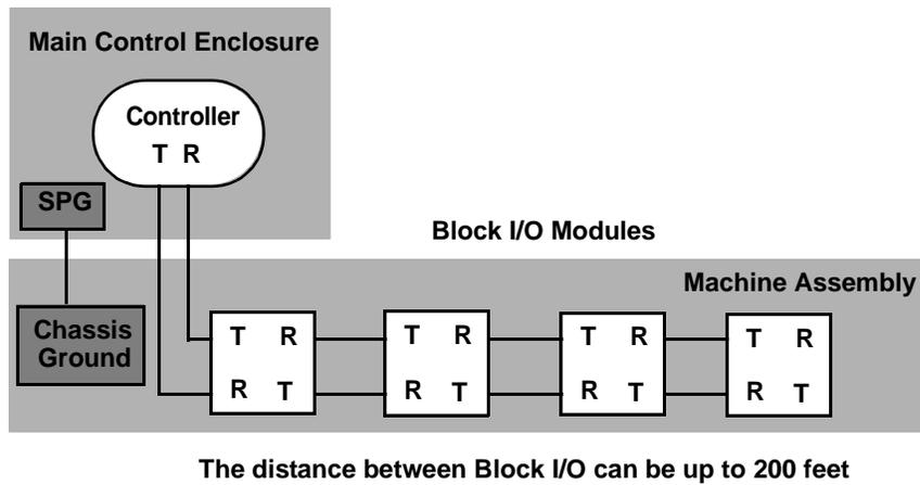
Figure 2-4 illustrates the distribution of the block modules around several sites that do not have the same common chassis ground. The chassis ground of each site should be connected to the SPG in the main control enclosure.
