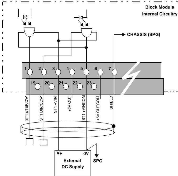
NOTE: As an alternative to an external DC power supply, you can use the +5V available on the block module. See insert for wiring.
