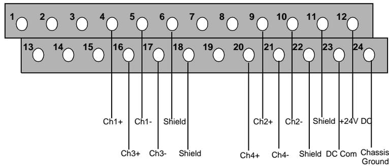
Each 4-20mA output channel is connected to a receiving device with twisted pair wires (see Figure 12-3). For extremely noisy environments, use shielded twisted pair wire.
