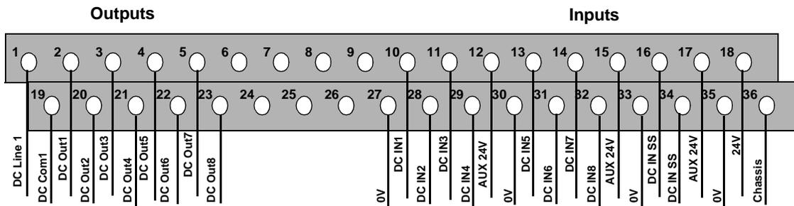
Typically, an external 24V DC supply is connected to pins 18 and 35.
