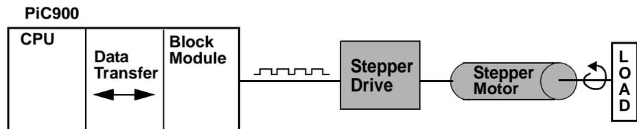
The block module controls the position, velocity, and acceleration of the stepper motor. The number of pulses generated by the block module provides distance information (steps) and the rate of these pulses provides velocity information (steps/sec). The rate of change of the pulse rate provides acceleration/deceleration information (steps/sec/sec).
