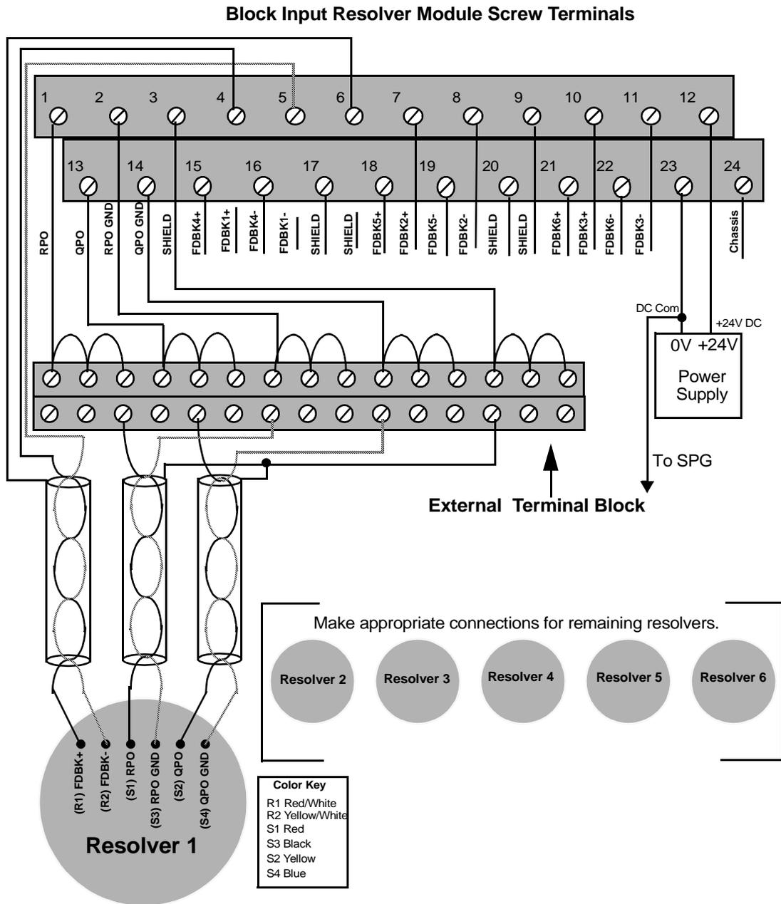
**NOTE:** If the count direction is incorrect after making the connections (i.e. clockwise rotation is counting down when it should be counting up), swap S1 with S3 or S2 with S4.
