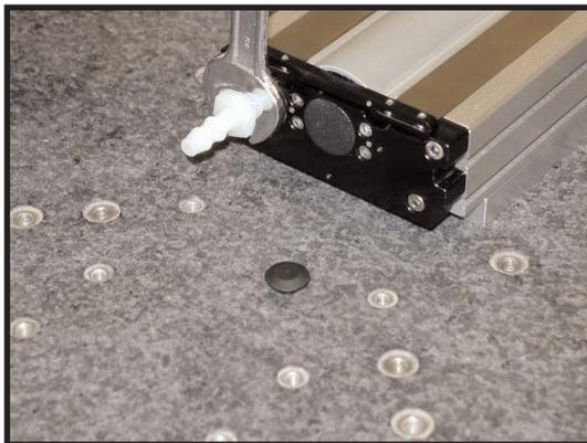
(4) Attach the 1/4" diameter tubing to the barbed end of the vent tube fitting.
