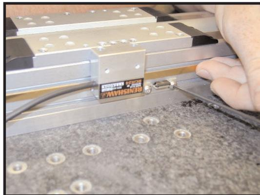
**Note:** The green light should flash red as the encoder readhead passes over the index mark.
