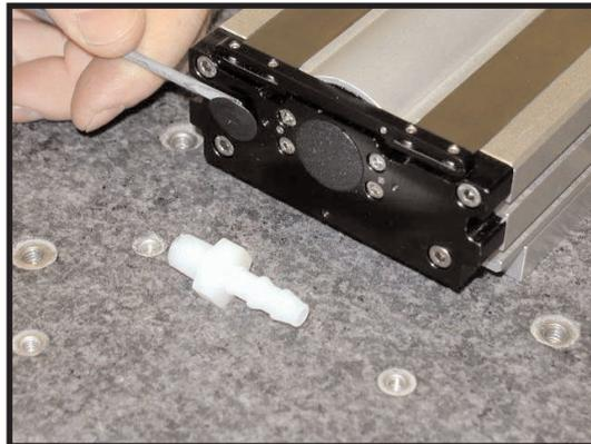
(2) Thread the NPT vent tube fitting into hole clockwise.
