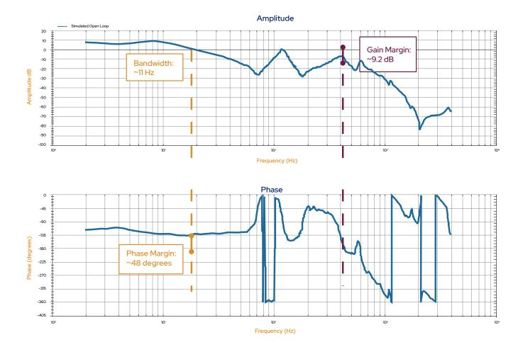
A 3-axis laser cutting machine was designed using the inertia matching approach for selecting the axis motors. A redesign was desired to reduce cost and improve performance of the machine. A review of the application requirements showed that alternate motor solutions could increase the system resonance point to allow additional gain and phase margins
