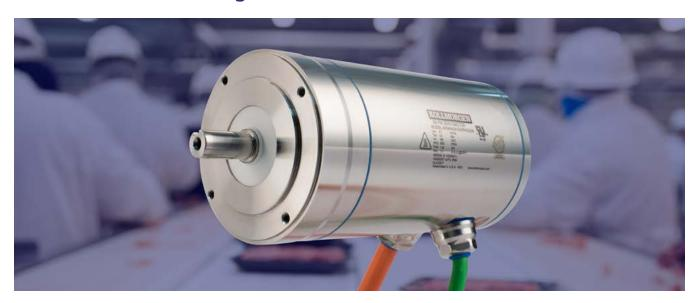
"The exterior of the AKMH is made entirely of stainless steel 316. In addition, it is completely polished and has a surface roughness better than 0.8 µm. All seals and O-rings also meet the strictest hygienic requirements. Even the motor type plate is laser engraved on the housing. The stainless steel Kollmorgen motors are the cream of the crop in the food packaging production."
