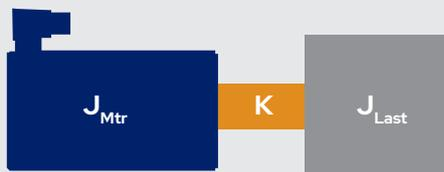
$$J_e = \frac{J_{Mtr} J_{Last}}{J_{Mtr} + J_{Last}} \quad F_{Antires} = \sqrt{\frac{K}{J_{Last}}} \quad F_{Res} = \sqrt{\frac{K}{J_e}}$$
