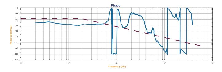
In a perfect system, we expect the Amplitude plot to be a straight negative slope, -20dB/decade. The Phase plot should start at -90° and drop at a negative slope from the point the amplitude crosses zero dB.
