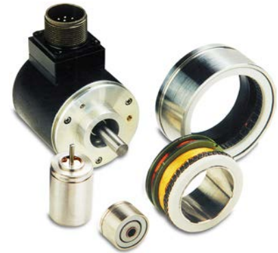
In a resolver, the position feedback signal is provided by the two sinusoidal signals, Sine and Cosine. A resolver-to-digital converter (RDC) encodes the analog sine/cosine waves into a digital signal that reports the motor's absolute position. Resolvers are durable and tolerate heat very well.
