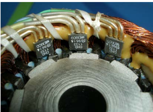
Hall effect devices are digital On/Off sensors constructed of semiconductor material used to sense the presence of magnetic fields. In brushless servomotors, they are used as position feedback when six-step commutation is employed. Six-step drives incorporate this feedback for crude velocity sensing or course positioning. With sinusoidal current drives, they are sometime used along with incremental encoder feedback to give a course power-up position indicator. In this image the sensors are integrated into the end-turns of the motor stator winding and are actuated by the rotor magnets.
