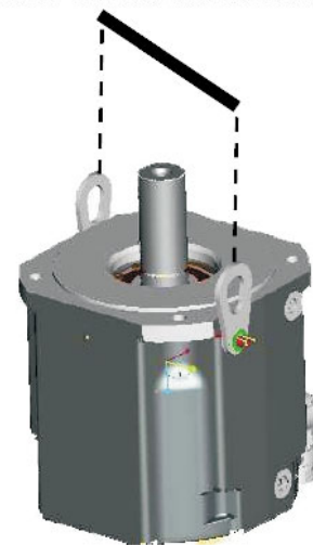
B2/ 2 x LIFTING BOLT PLUS LIFTING BEAM
