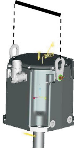
B3/ 2 x LIFTING BOLT PLUS LIFTING BEAM
