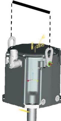
B3/ 2 x LIFTING BOLT PLUS LIFTING BEAM
