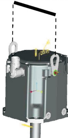
B3/ 2 x LIFTING BOLT PLUS LIFTING BEAM
