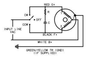
Red goes to Resistor White goes to Neutral (center tap of the two coils) Black goes to Capacitor.
