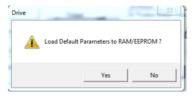
After reset, the Drive software will UPLOAD the parameters showing indication of the upload and then proceeding with the Drive software being online ( and synchronized with the drive parameter values. An indication the drive is reset to factory default is the motor is undefined ( "NN").
