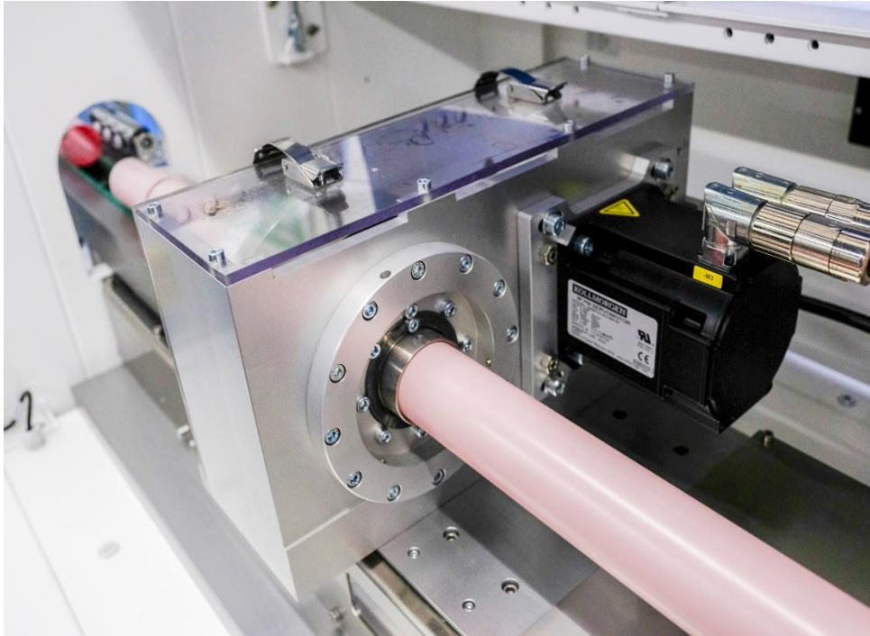
The blades driven by AKM servo motors work with precisely regulated centrifugal forces.
