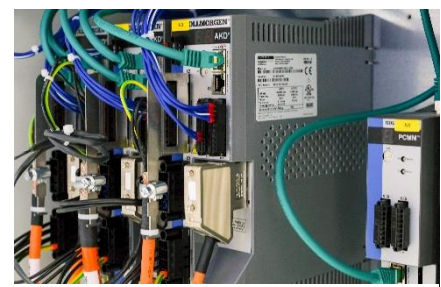
With the combination of the PCMM Motion Controller and AKD servo drives, Breyer has a compact and high-performing motion control combination.
