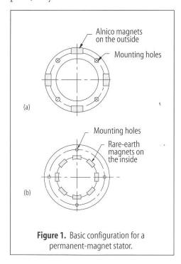
ing on the exposed end of a shaft. Mounting features for this arrangement include round or square flanges or tabs on the stator housing.
