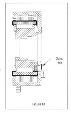
The pole-piece clamp type, as seen on the T-18002 motor, locks the armature to the field at the air gap by forcing a number of movable field pole-pieces radially inward until clamping action takes place (see Figure 11). After installation of this type motor, the clamping set screws are loosened, and the pole-piece stud nuts are retightened to secure the pole-pieces in their proper position.
