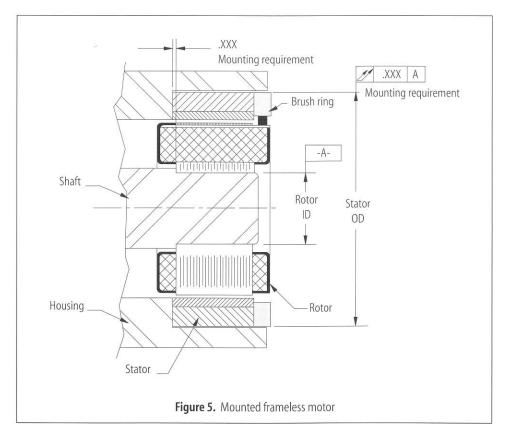
drawing. (See Figure 5.) If this axial tolerance is exceeded, the brushes may fall off the commutator or ride into the rotor stack. If axial deflections or tolerance buildups do not allow for this mounting dimension, call the factory for advice.
