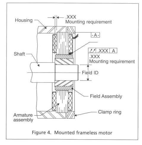
Bonding the rotor to the shaft is the most common method of rotor mounting. As with the stator, a key and keyway can be applied for added strength.
