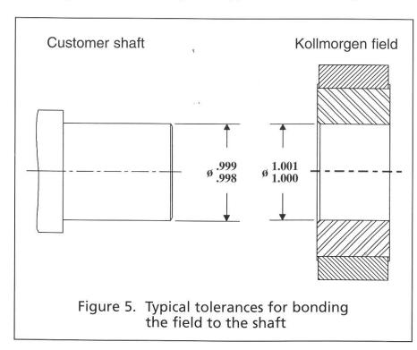
outline drawing (see Figure 4). This toleranced dimension must be held to maintain optimum motor performance. If axial deflections or tolerance buildups do not allow for this mounting dimension to be held, call the factory for advice.
