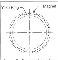
Figure 3. Basic configuration for a field assembly.
