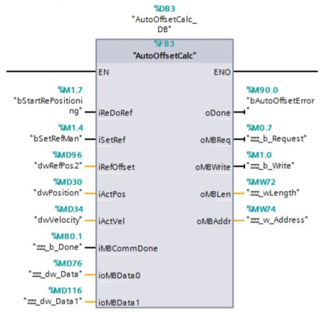
In the data bloc all variables have to be set as **retain**, to enable a recalculation of the position after a power down situation.
