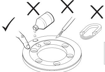
WARNING: Magnetic rings should not be exposed to magnetic field densities higher than 50 mT on its surface. Magnetic fields higher than 50 mT can damage the ring.
