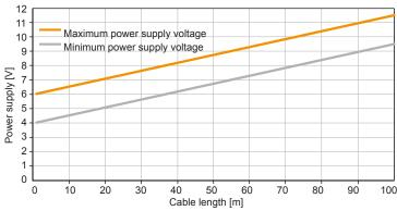
For cables longer than 5 meters input voltage on the cable must be adjusted so the voltage drop is taken into account.
