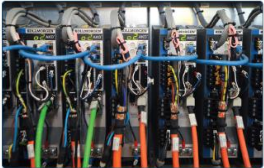
The AKD Servo controller with EtherCAT communication - the compact design makes the cabinets smaller.
