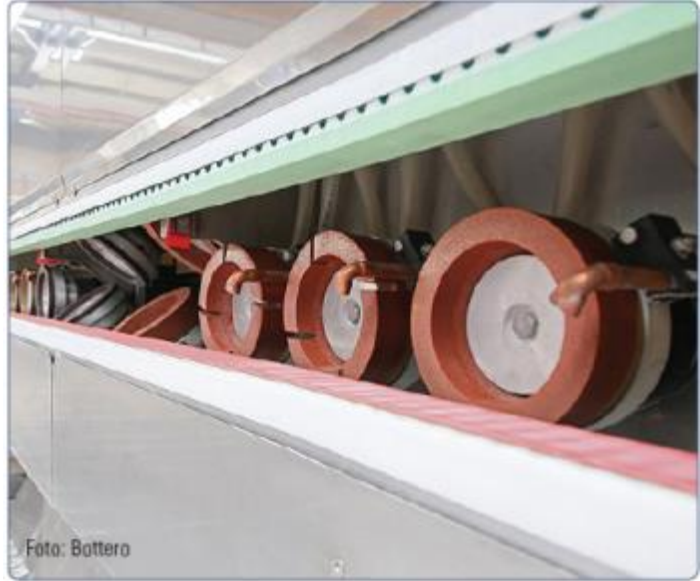
KOLLMORGEN drives allow the precise positioning of the glass sheets and the drive of grinding wheels.
