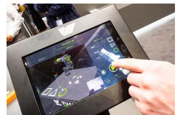
Specialist knowledge is no longer required to program the robot: 3D visualization, making use of the potential of augmented reality, is revolutionizing the commissioning process.
