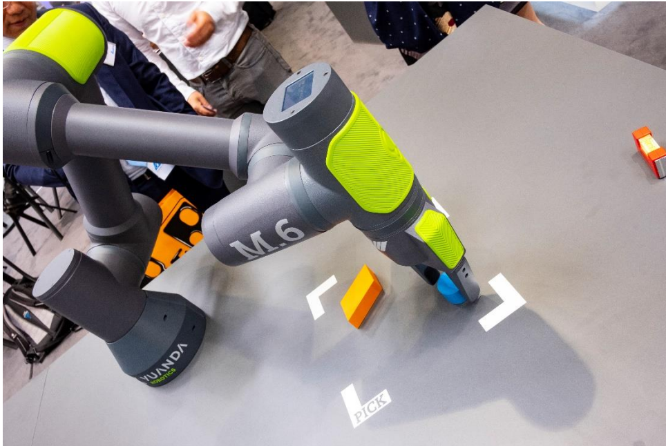
The M.6 has an average carrying capacity of 6 to 8 kg (M) and consists of six drive units (6).
