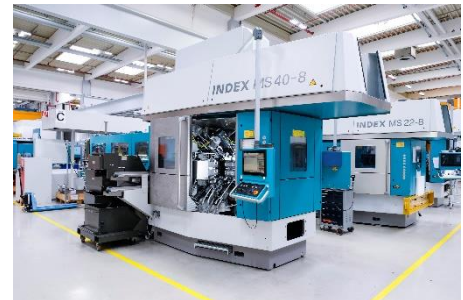
The MS40C-8 from Index is designed as a CNC multi-spindle machine for large and small production batches.
