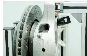
IMS Gear tests the long-term behavior of parking brakes on brake test benches. The drives must show excellent control characteristics for this.
