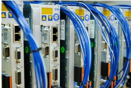
EAT uses the S700 KOLLMORGEN servo controller for precise and complex control tasks.
