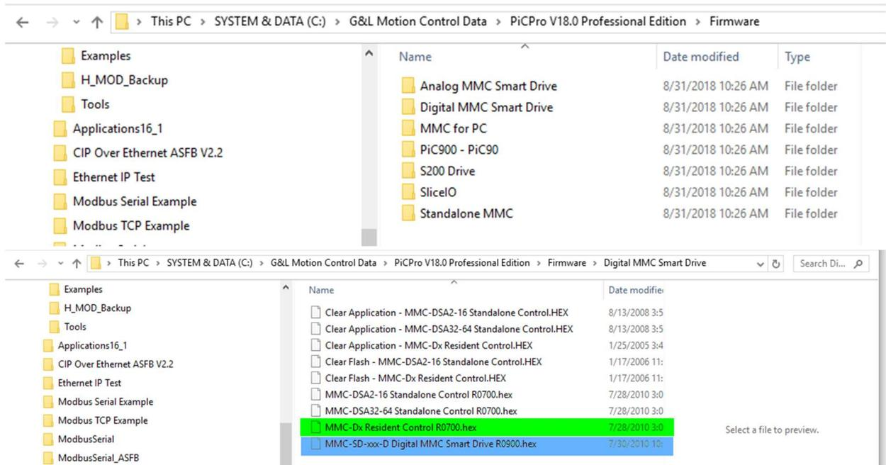
For the installed version of PicPro the compatible firmware versions are shown above ( R0700 for the drive resident control and 0900 for the digital MMC drive.
