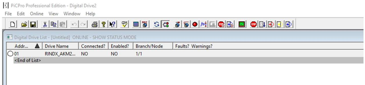
Highlight the drive desired with your mouse cursor and then double-click the highlighted drive in the list to open the Digital Drive
