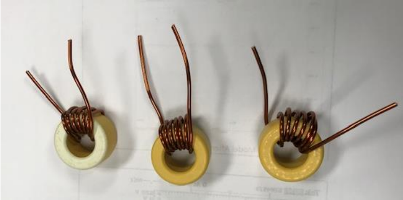
Figure 18: Differential mode cores wrapped with 6 turns over Micrometals 26 powdered iron for 50uH each phase, 100uH in series.
