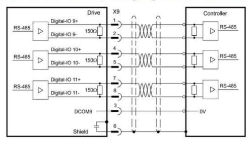
Differential RS485 General I/O Wiring Diagram with a Controller or PLC
