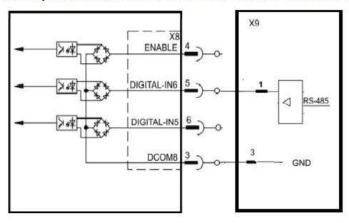
Differential RS485 Wiring Diagram connectioning Dout 9 to Din 10
