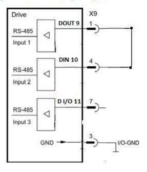
The DOUT9 and the DIN10 are both referenced to the same I/O-GND.
