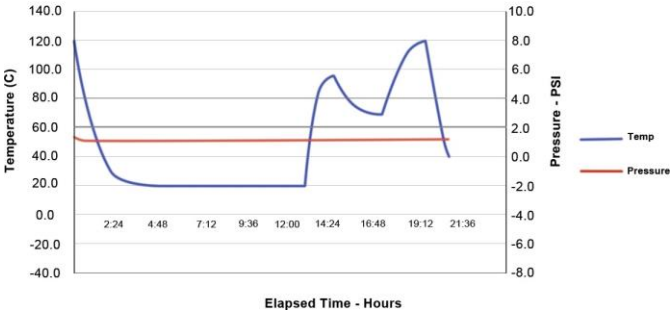
Sample #8 - Pressure/Vacuum Excursion vs Temperature - Open Systems (Vented Cable)
