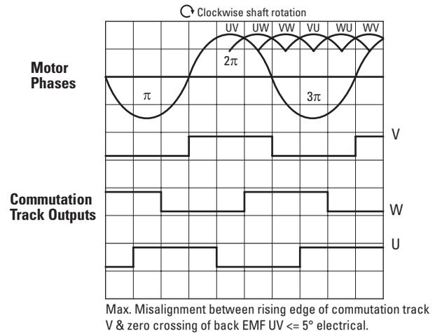
Max. Misalignment between rising edge of commutation track V & zero crossing of back EMF UV  $\leq 5^\circ$  electrical.
