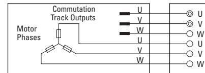
Output Comm: Open Collector W 2.2 k OHMS
