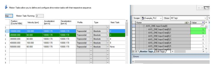
In some cases the programmer may want to add code to validate that the position is at the final target position based on feedback position and the in position window status before declaring the chain of moves complete but this is up to the programmer.
