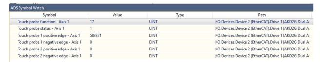
On rising edge of DIN 1 the Touch probe status-Axis 1 changes to 1 to 3 (touchprobe 1 is enabled and new positive edge position store on touchprobe 1) and a new positive edge is captured.
