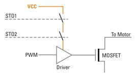
This implementation of the STO works with negative logic, deactivating the power stage by default. In order to activate the power stage, and therefore allow the motor to operate, two differential inputs must be energized. These inputs activate two optocouplers that enable the power supply of the Half-Bridge Gate-Drives that control the power stage. If the STO inputs are not energized, the transistors of the power stage are turned off because the Half-Bridge Gate-Drives are turned off.
