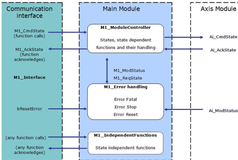
**Figure 6-36:** Context Diagram for Main Module
