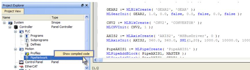
**Figure 4-14:** Display Source Code of the Pipe Network
