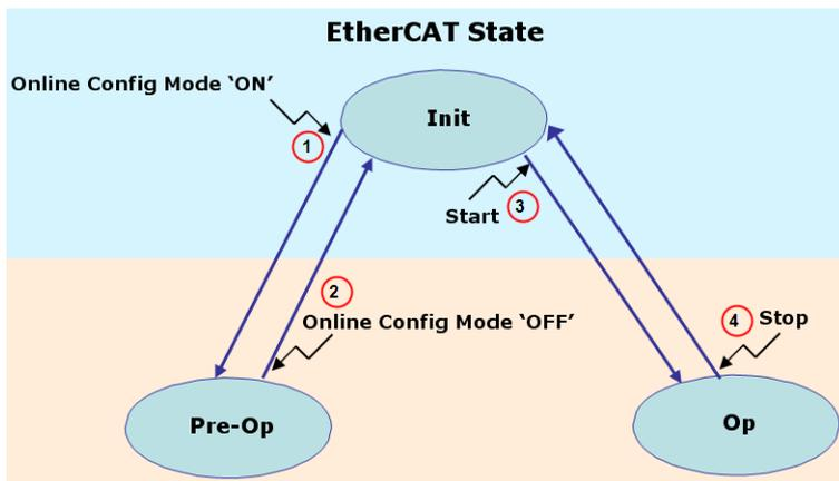
**Figure 9-34:** AKD Configuration According to EtherCAT State
