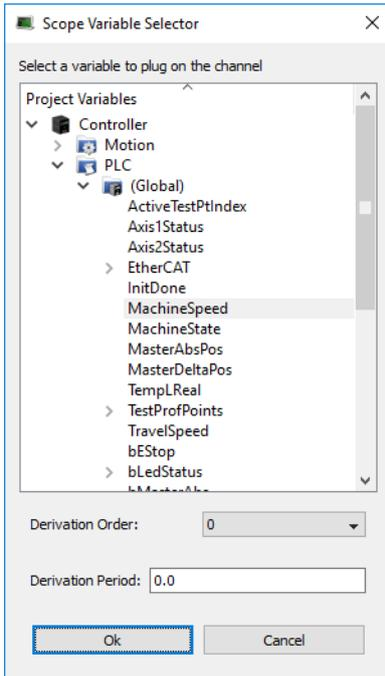
**Figure 5-56:** Using the Variable Selector to choose a variable to be mapped in the Oscilloscope
