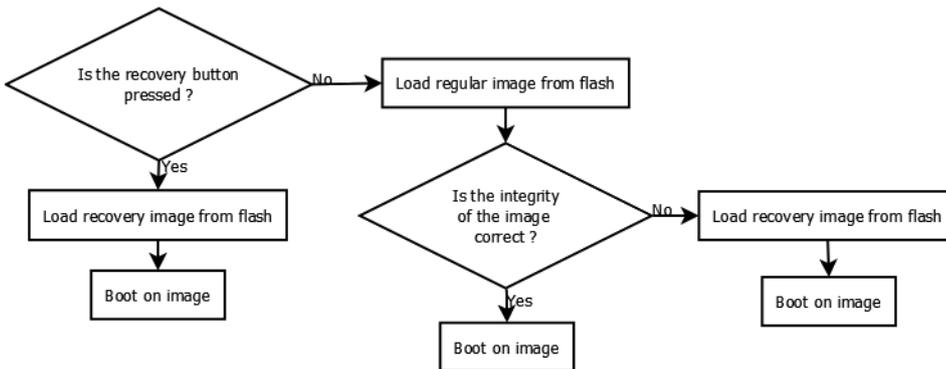
**Figure 5-2:** AKD PDMM and PCMM Flow
