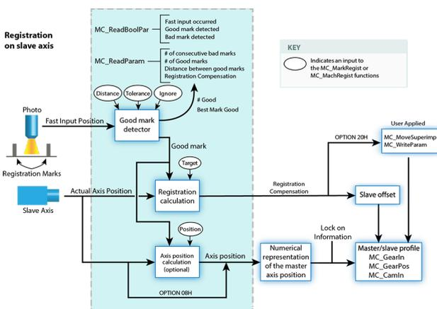
This "Registration" (→ p. 604) image is an example of a printing application using registration.
