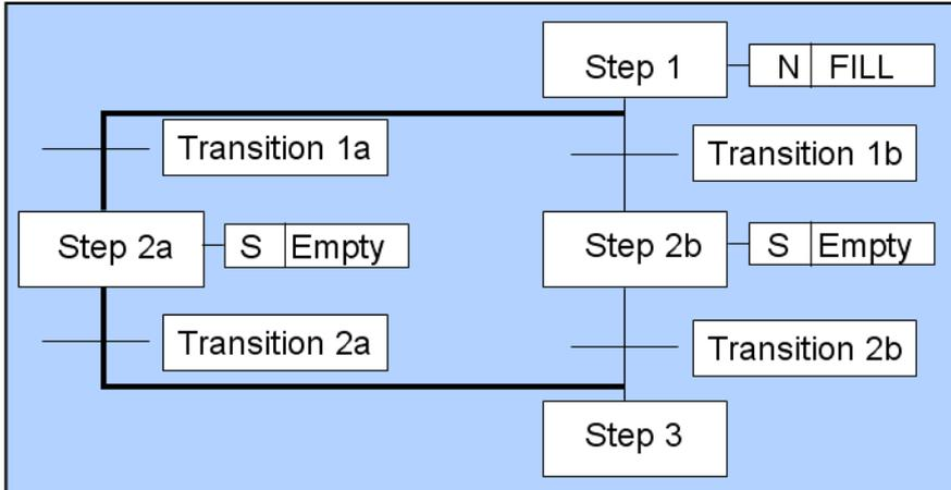
**Figure 9-1:** Example of a Parallel Sequence in SFC
