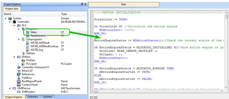
Figure 6-57: PLCopen Template with ST - Main
