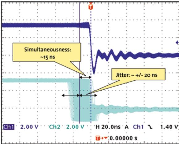
**Figure 9-22:** Synchronicity and Simultaneousness
