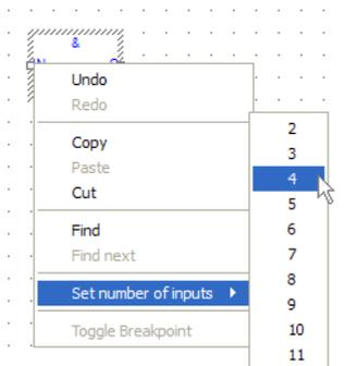
**Figure 4-31:** Set the Pins Number of the Block
