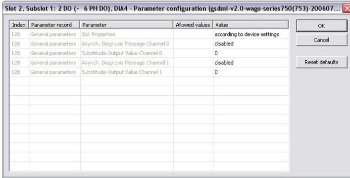
Figure 6-29: Example of configuring sub-modules.
