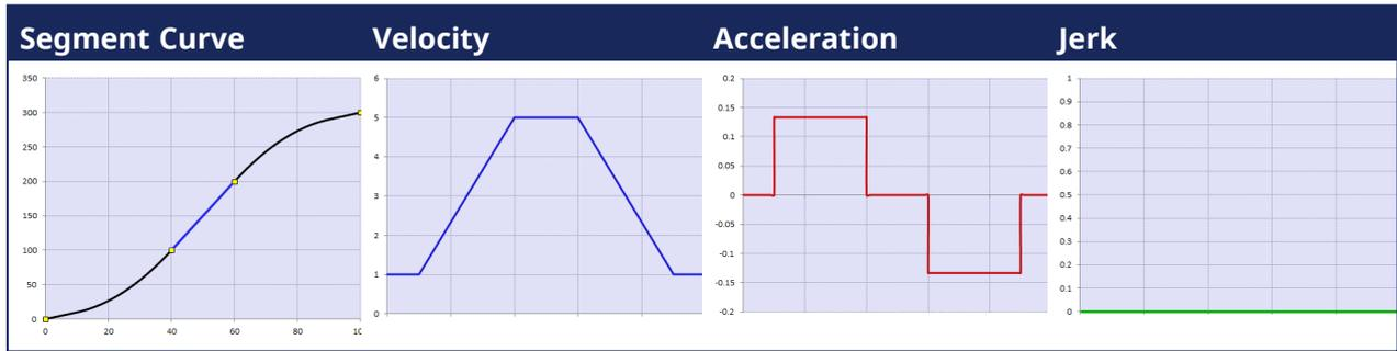
In the example shown, the blue line represents the linear (constant velocity) part of the segment, while the black lines represent the parabolic (constant acceleration) parts of the segment.
