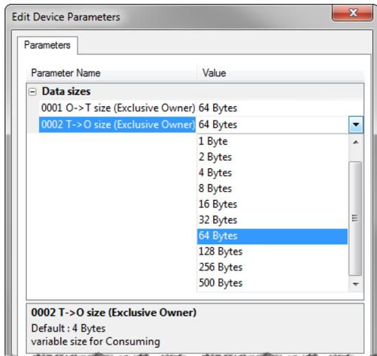
**Figure 6-27:** Example of setting byte sizes in a third-party Network Configurator.
