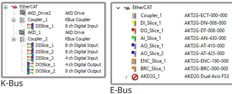
**Figure 4-103:** EtherCAT Network - Logical View
