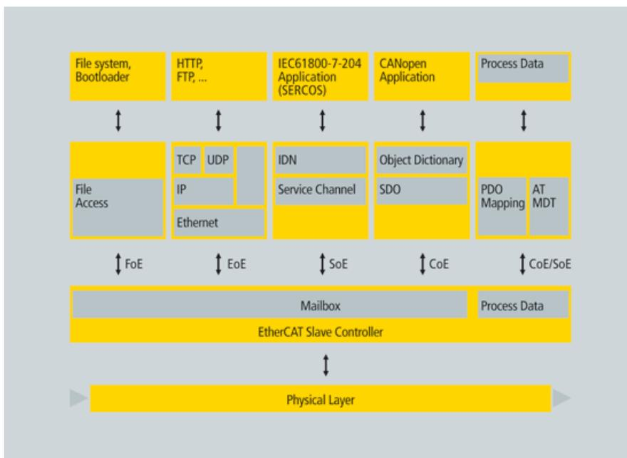
**Figure 9-26:** Several Device Profiles and Protocols can Coexist
