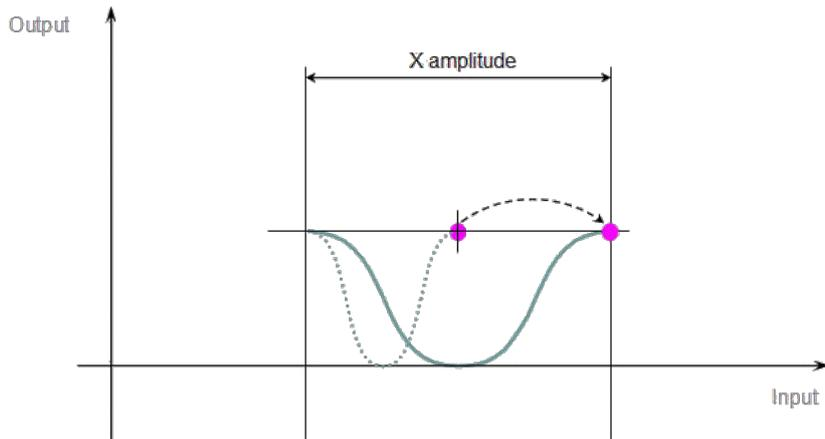
**Figure 4-42: CAM Profile Transformation - Step 2**
