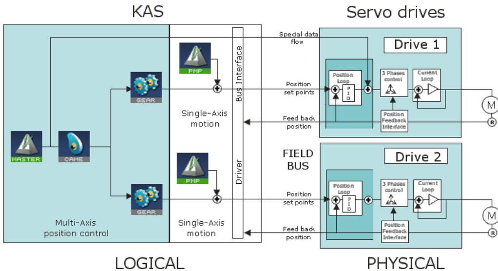
**Figure 9-4:** Hardware Organization of Motion Functions
