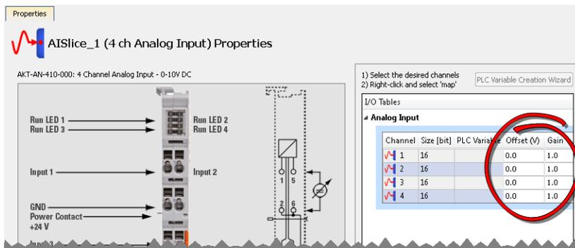
Figure 4-99: Analog Input Properties
