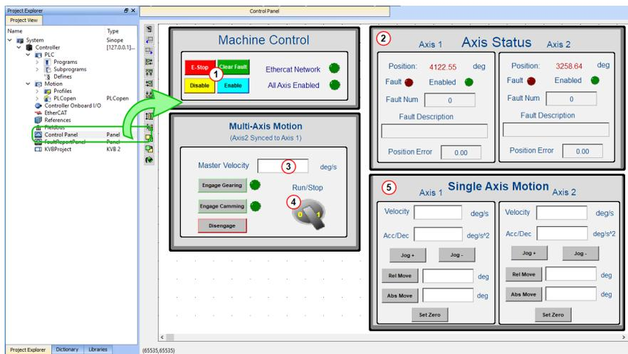
Figure 6-59: PLCopen Template - Control Panel
