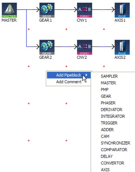
Figure 4-4: Pipe Network - Add Pipeblock
