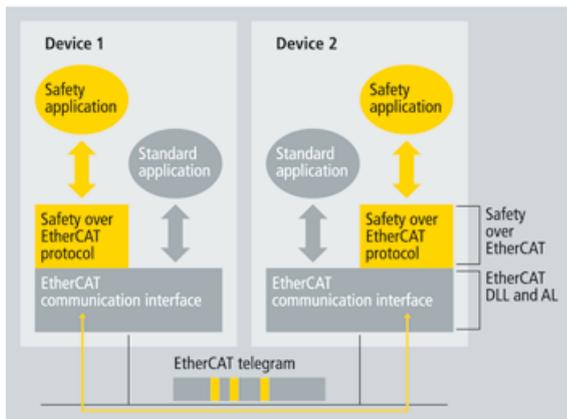
**Figure 9-24:** Safety over EtherCAT Software Architecture
