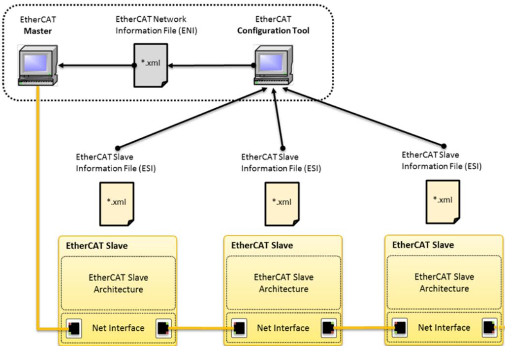
**Figure 9-29:** EtherCAT Network Architecture <sup>1</sup>
