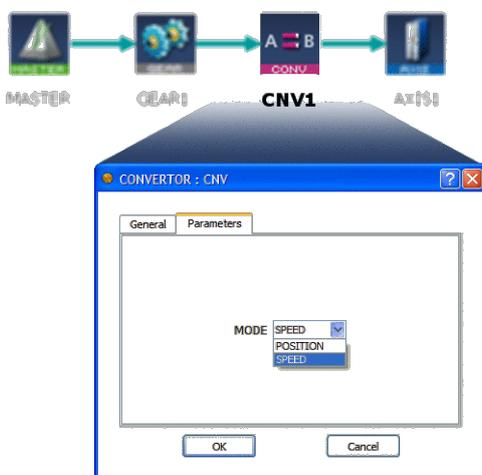
**Figure 9-9:** Change the Mode of Converter Block to SPEED (not POSITION mode).
