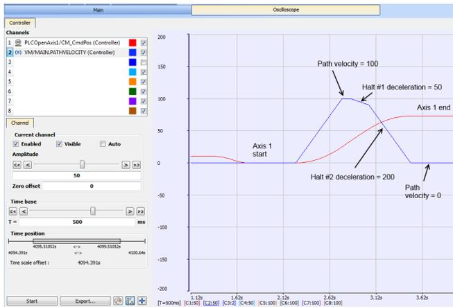
**Figure 6-12:** Oscilloscope Representation of linear coordinated move with a MC\_GrpHalt command called twice
