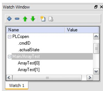
**Figure 3-11:** Watch Window - Accessing Arrays
