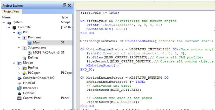
Figure 6-51: PLCopen Template with ST - Main
