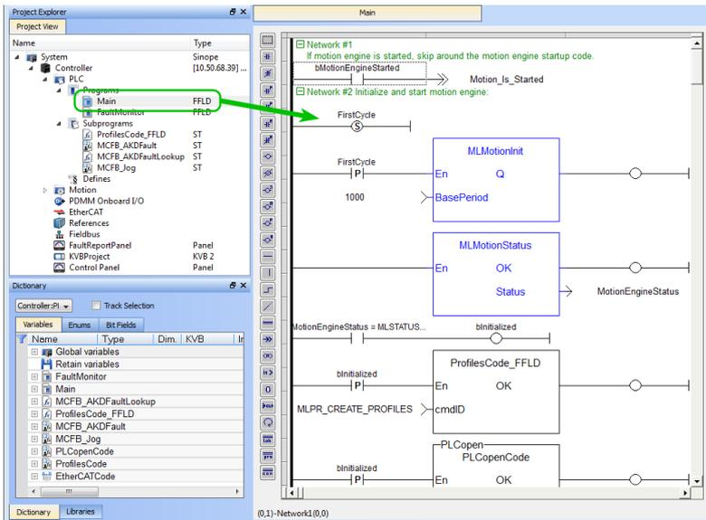
Figure 6-64: PLCopen Template with FFLD - Main
