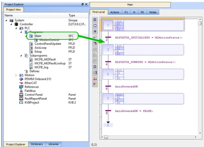
**Figure 6-52:** PLCopen - Template Main
