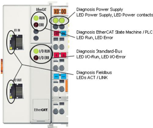
**Figure 10-2:** ETHERCAT Coupler Diagnostic LEDs
