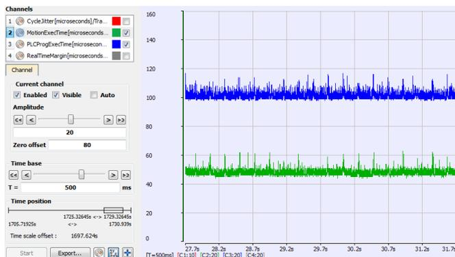
Figure 5-68: MotionExec and PLCProgExec Times
