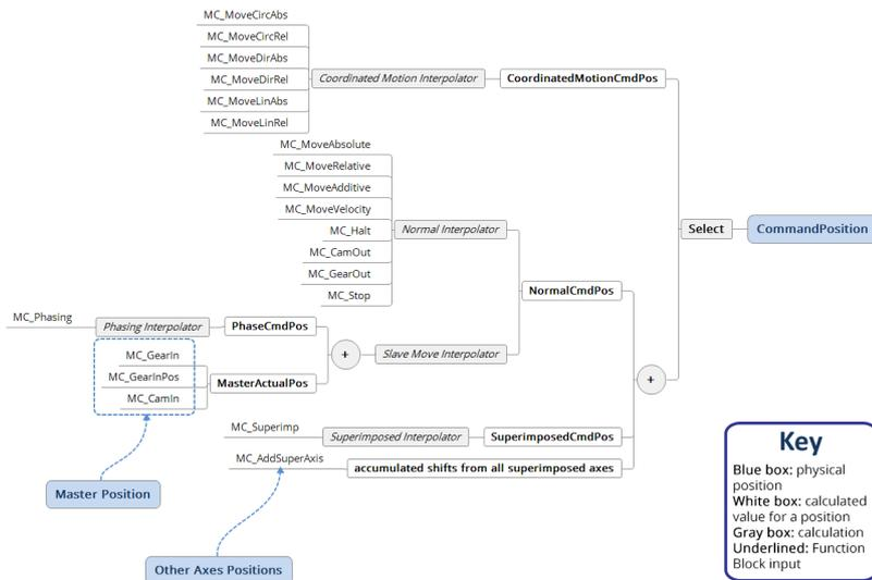
**Figure 9-14:** Calculated PLCopen Axis Position Data
