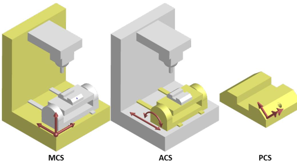
Figure 6-1: Examples of CS types on a machine and part.
