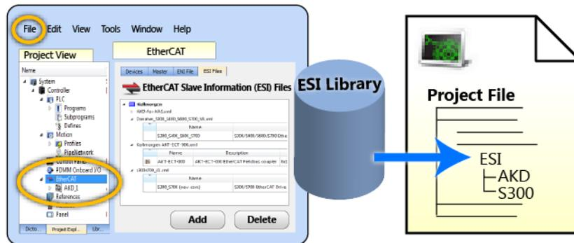
**Figure 4-110: Saving** — When a KAS project is saved, a copy of the ESI file(s) is included in the project file.
