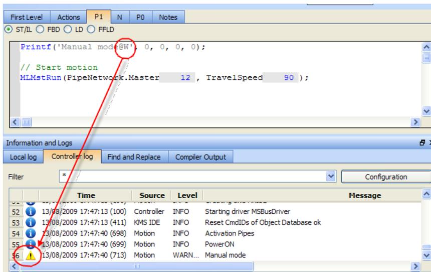
**Figure 4-56: Customizing Output for Printf**
