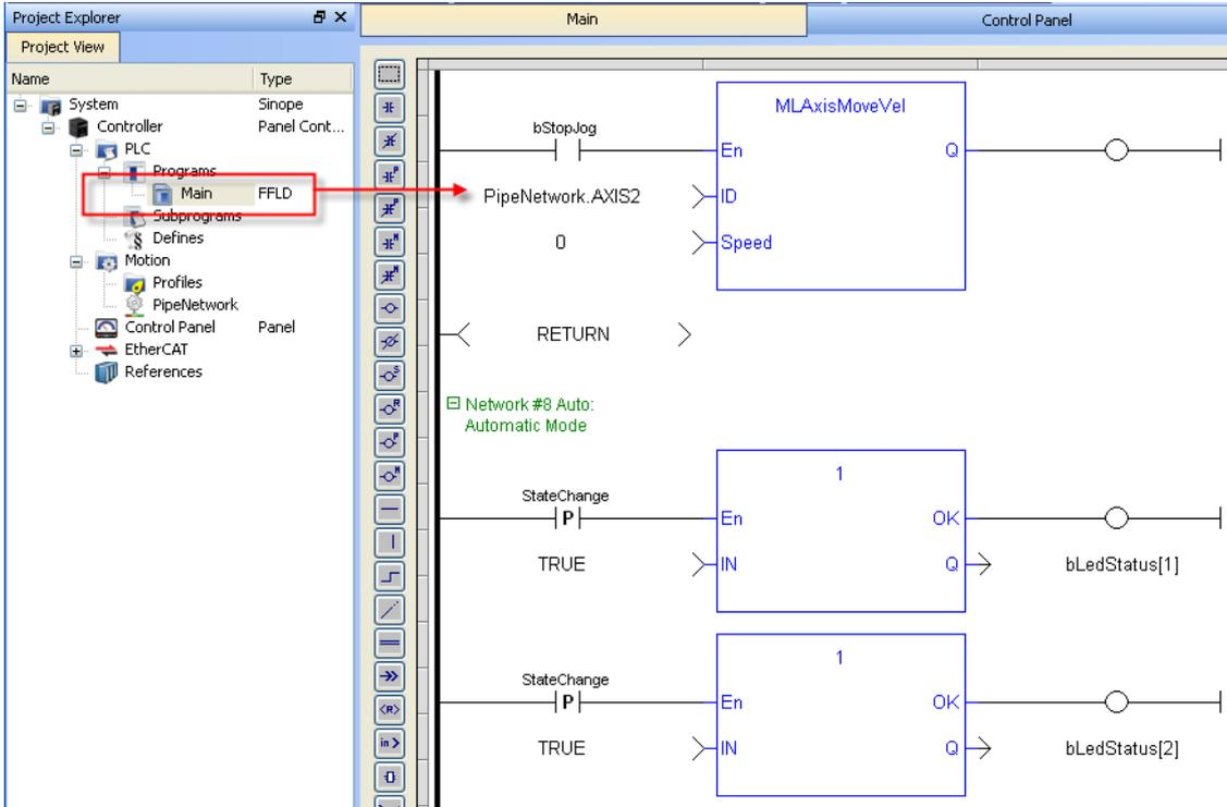
Figure 6-49: PN Template with FFLD - Main
