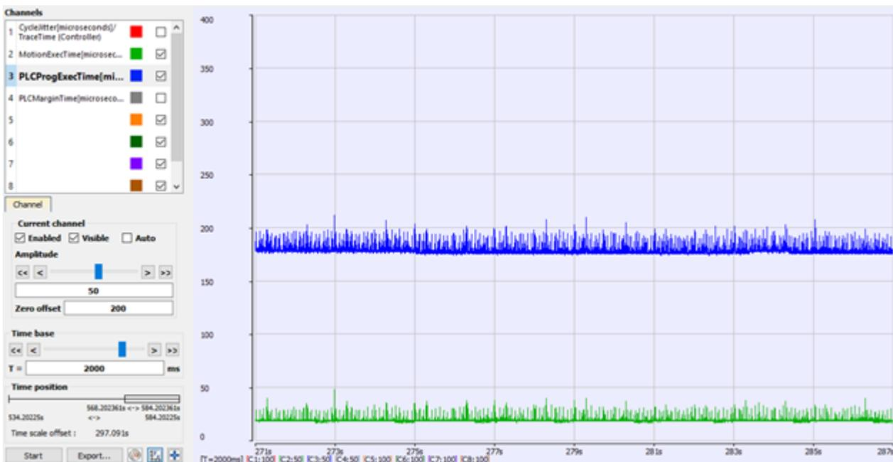
**Figure 5-77: MotionExec and PLCProgExec Times**
