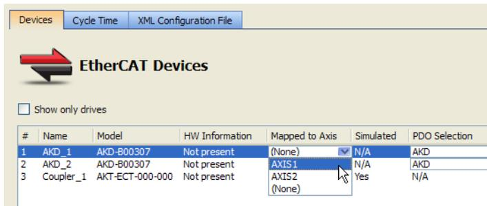
**Figure 4-10:** Pipe Network - Mapping Axis to Drive
