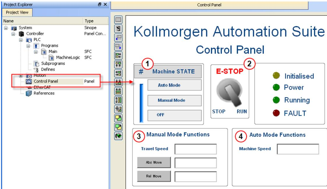
Figure 6-40: PN Template - Control Panel
