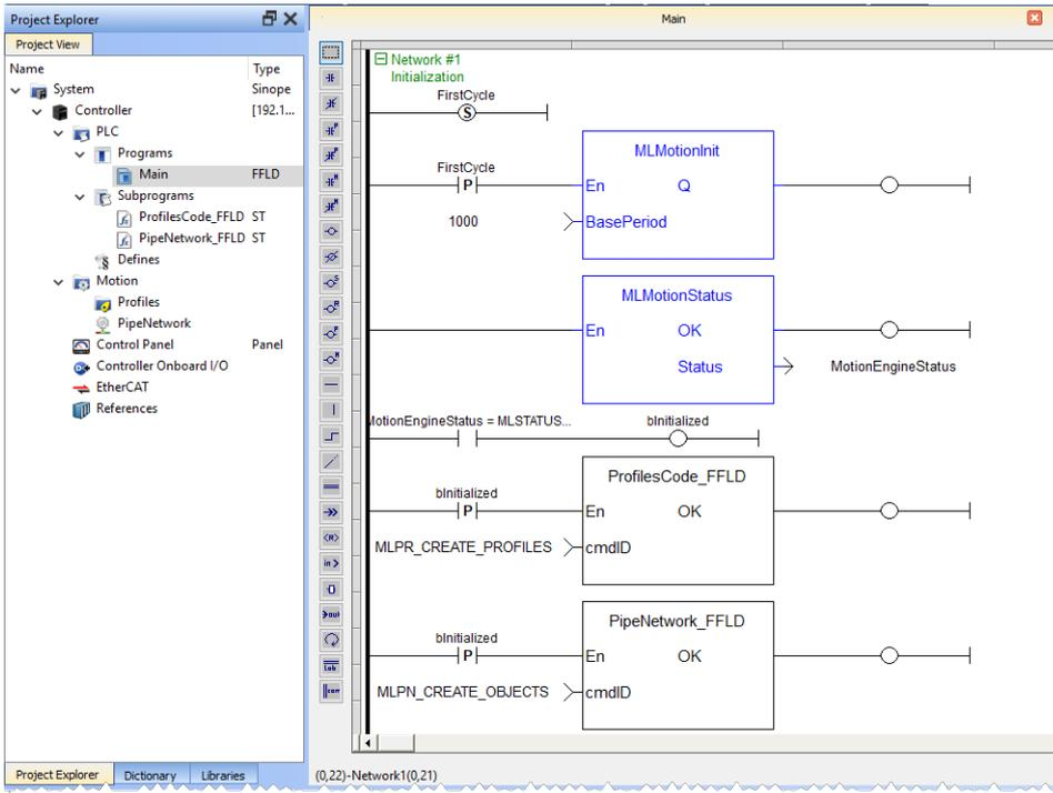
Figure 6-38: PN Template with FFLD - Main
