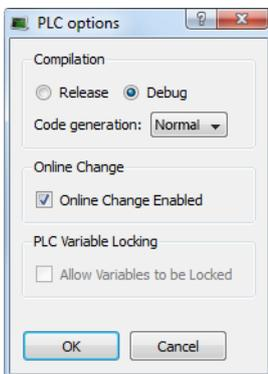
**Figure 4-53:** PLC Options - Debug Compiling Mode
