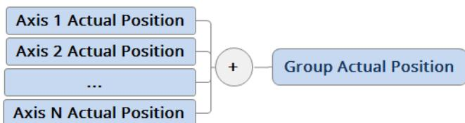
**Figure 9-13:** How **Actual Position** is Calculated
