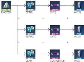
The Pipe Network is used to create a high-performance motion algorithm which is tightly integrated to the PLC program with motion library function blocks.
