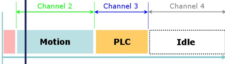
Figure 5-50: AKD PDMM or PCMM - Single Core Controller, Motion, PLC and Real Time Margin Time Calculations
