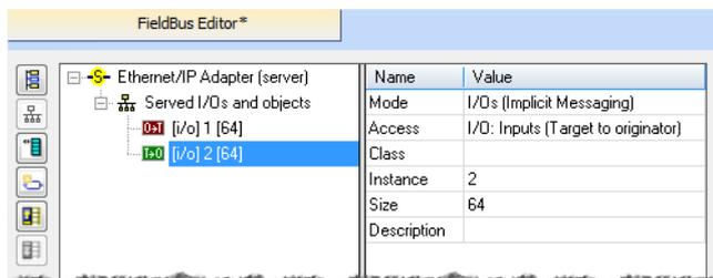
**Figure 6-28:** Example of setting byte sizes in the KAS-IDE Fieldbus Editor
