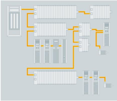
**Figure 9-21:** Flexible Topology: Line, Tree, or Star
