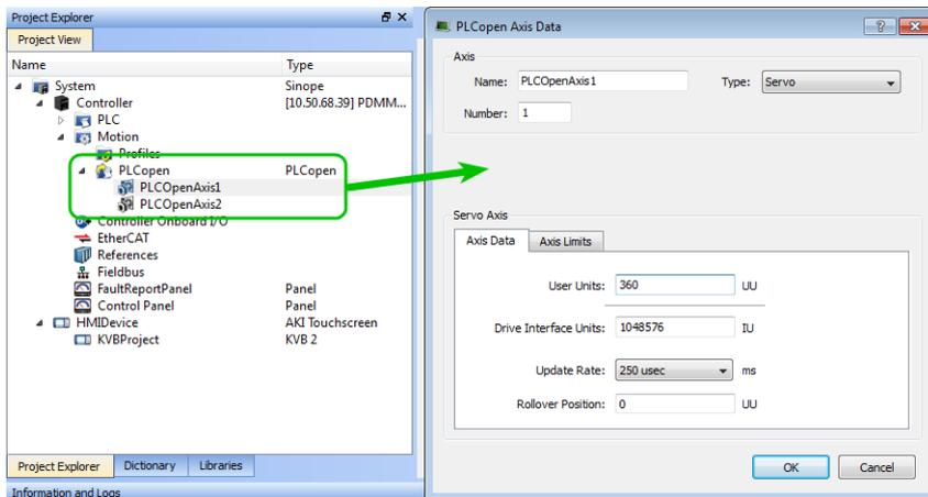
**Figure 6-63:** PLCopen Template - Motion
