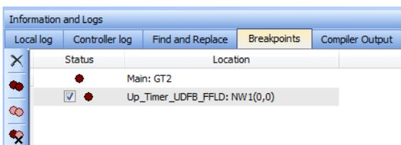
**Figure 3-8:** Example of a breakpoint (*Main: GT2*) set in an SFC program.
