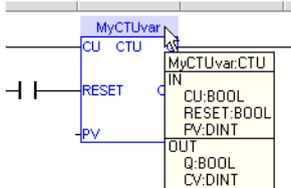
**Figure 4-73:** Tooltip on Variable
