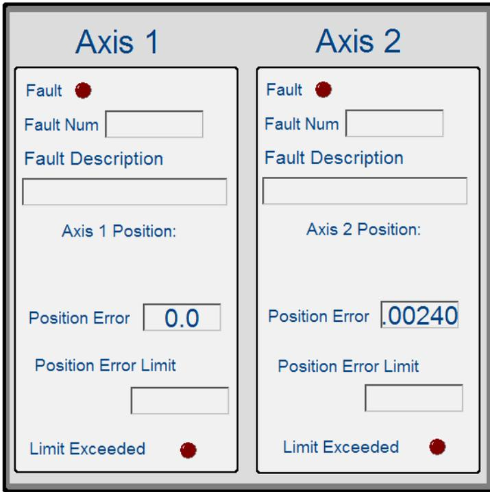
**Figure 6-60:** PLCOpen Template - Fault Report Panel
