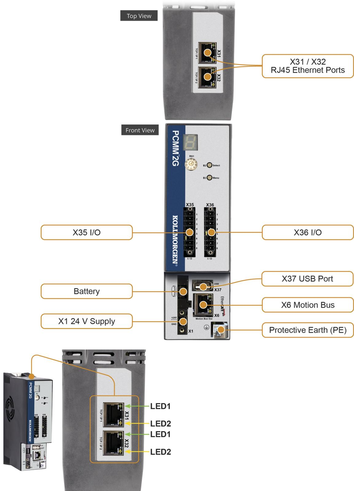
**Figure 4-117:** PCMM2G Hardware Connections
