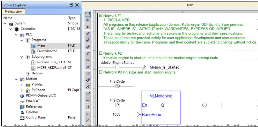
Figure 6-50: PLCopen Template with FFLD - Main
