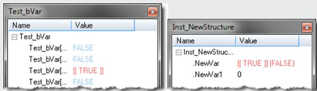
The variable locking feature can be enabled or disabled via the PLC Options device toolbar button. If enabled, the Lock and Unlock buttons are accessible:
