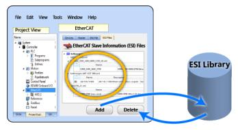
**Figure 4-109: Adding/Deleting** — Adding or deleting an ESI file from the KAS-IDE affects KAS's internal library of ESI files.
