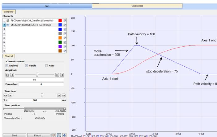
**Figure 6-13:** Oscilloscope Representation of linear coordinated move with a MC\_GrpStop
