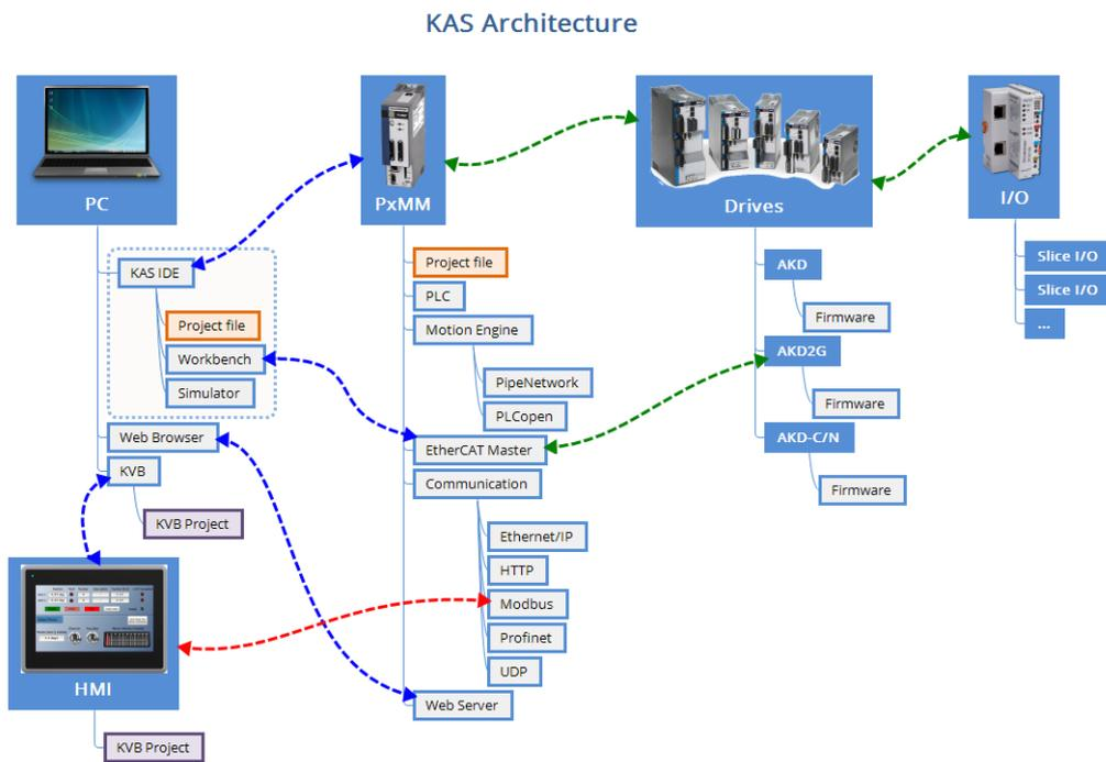
Figure 2-6: Architectural view of KAS components
