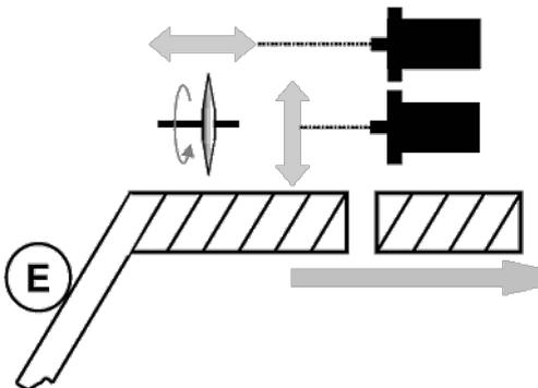
**Figure 2-2:** Spring Winding
