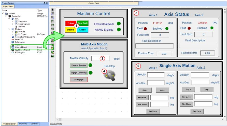
Figure 6-61: PLCopen Template - Control Panel
