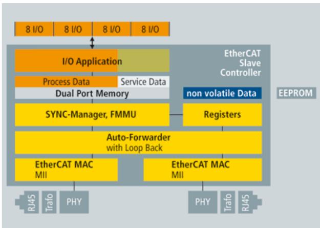
Figure 9-31: Slave Hardware: FPGA with direct I/O
