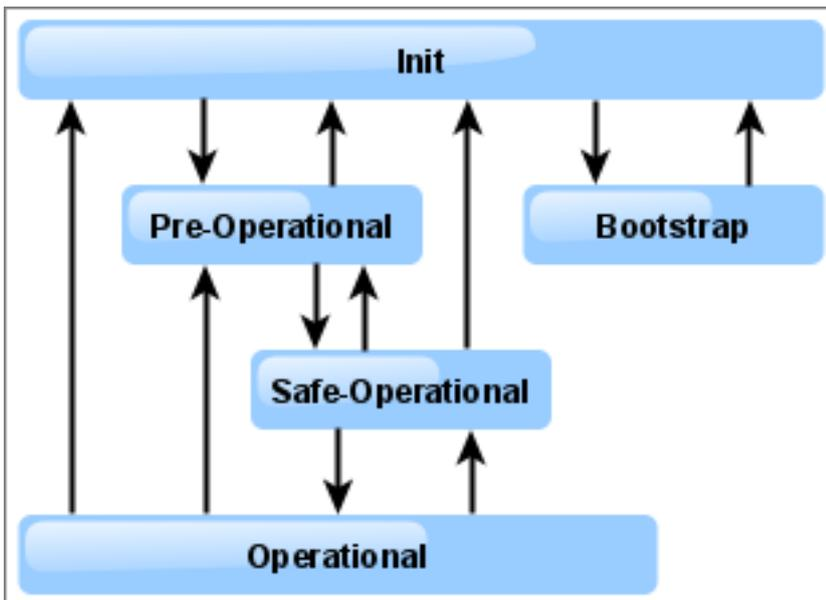
Figure 9-32: EtherCAT State Machine
