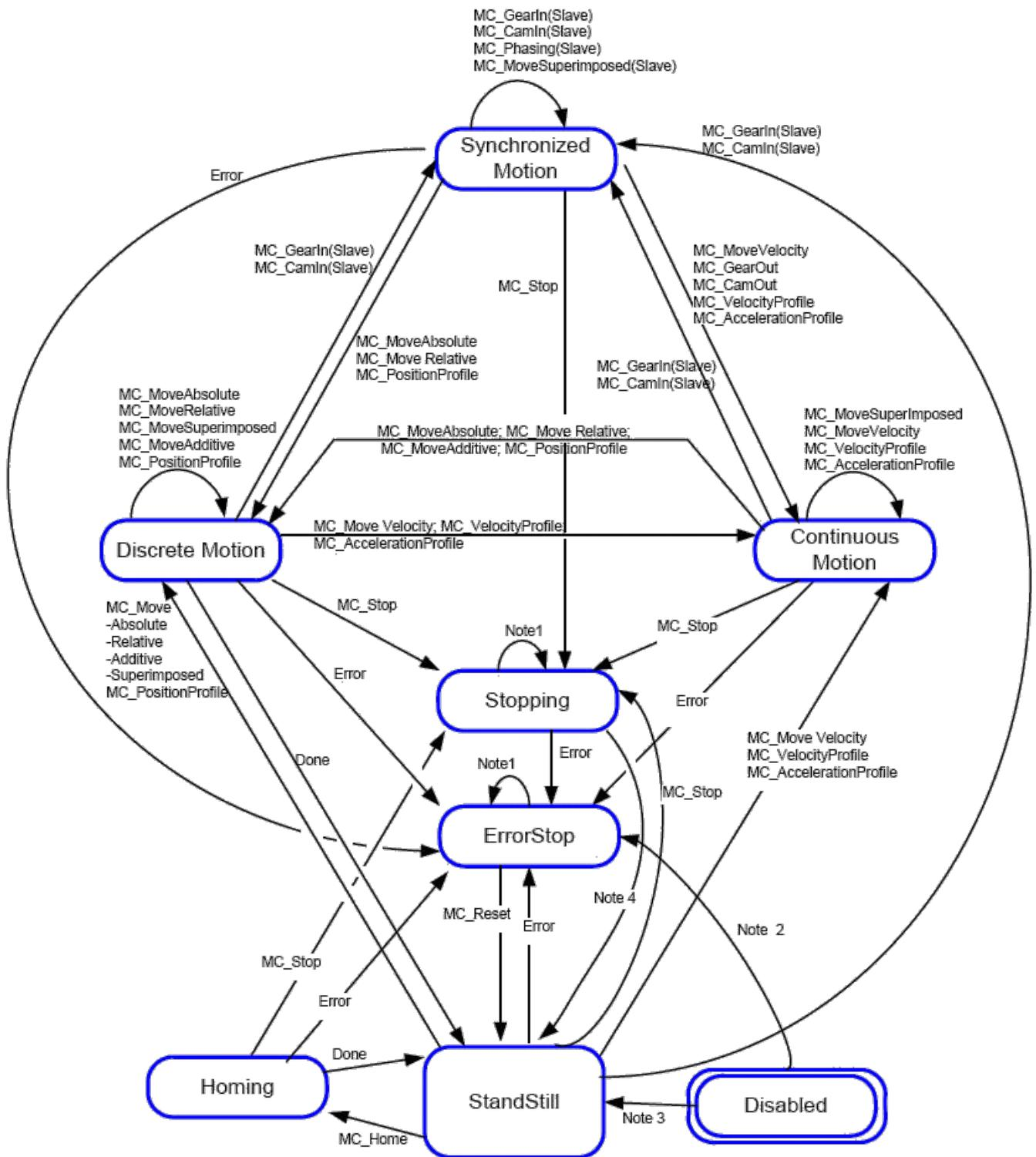
**Figure 9-18:** Motion State Machine (PLCopen)
