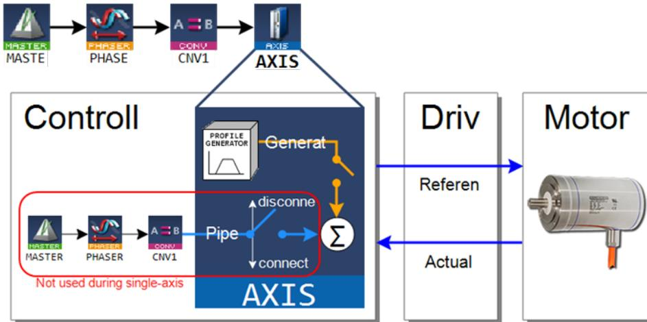
Figure 9-10: Axis Pipe Block Positions
