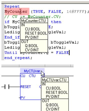
Figure 4-71: Tooltip on Variable
