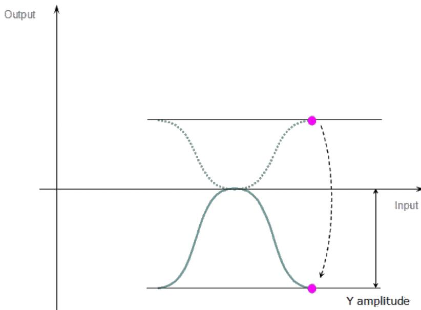
**Figure 4-43: CAM Profile Transformation - Step 3**
