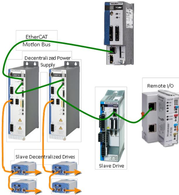
**Figure 4-102:** EtherCAT Network - Physical View
