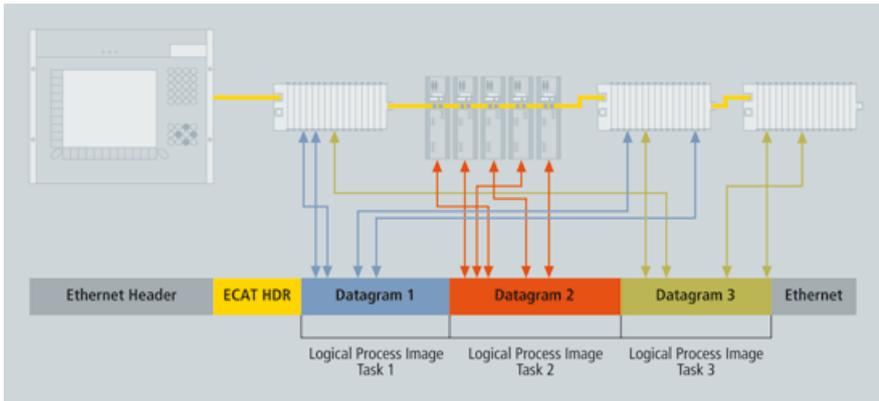
**Figure 9-20:** Process Data is Inserted in Telegrams
