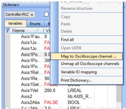
**Figure 5-57:** Plugging a Probe from the Dictionary
