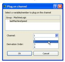
Figure 4-61: Plugging a PLC Variable - Parameters
