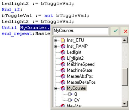
Figure 4-70: Autocompletion
