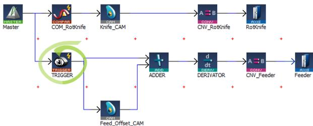
**Figure 6-22:** Example of using a Pipe Network Trigger block for position capture.
