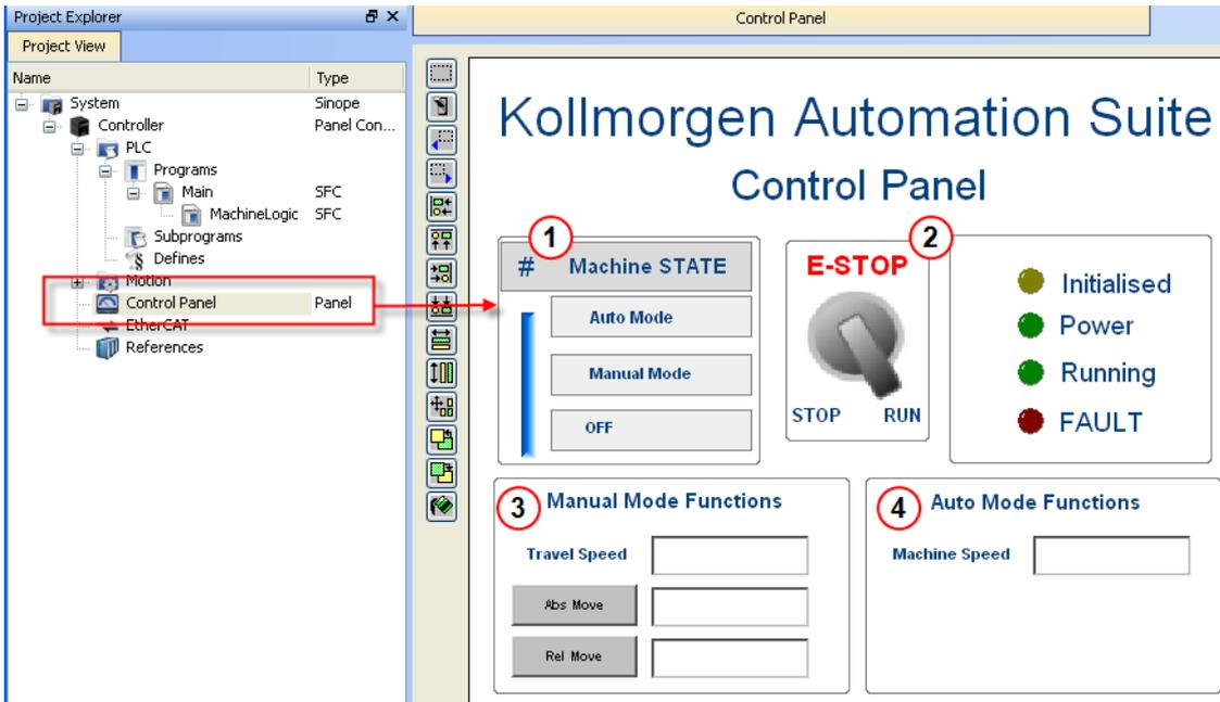
Figure 6-47: PN Template - Control Panel
