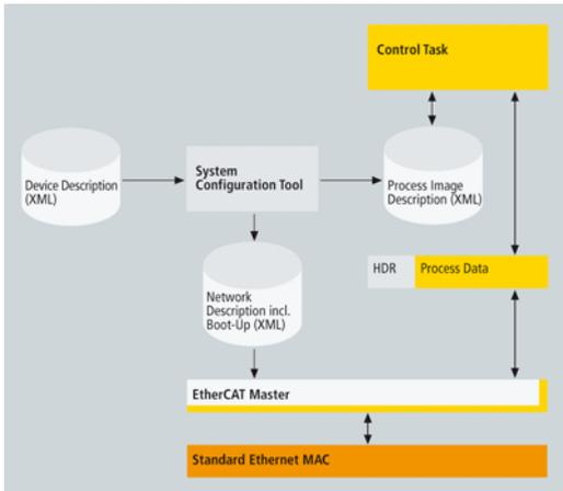
**Figure 9-28:** Structure of EtherCAT Master Implementation
