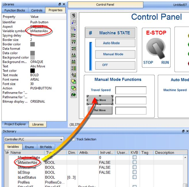
Figure 5-38: Map Variables to a Control Panel Control in the Graphical Editor
