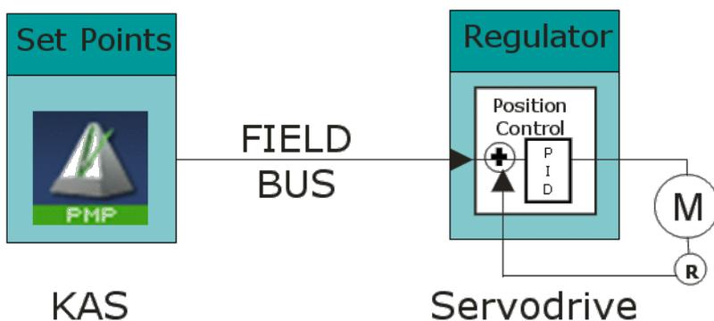
Figure 9-2: Regulation with Remote Drive
