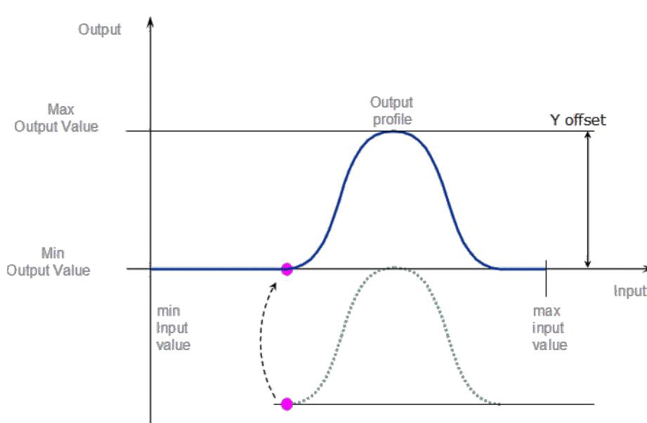
**Figure 4-44:** CAM Profile Transformation - Step 4
