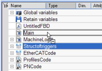
**Figure 4-87:** Create an Instance of the Structure
