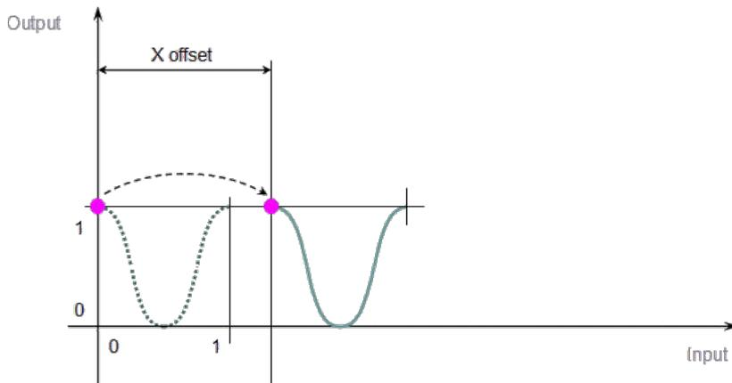
**Figure 4-41: CAM Profile Transformation - Step 1**
