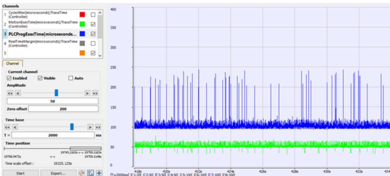
Figure 5-73: MotionExec and PLCProgExec Times
