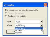
Figure 4-89: Define Type and Scope of the Variable
