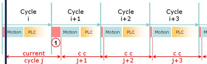
**Figure 5-48: Cycle Time Calculation**
