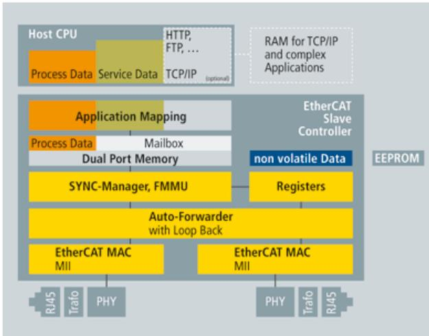
Figure 9-30: Slave Hardware: FPGA with Host CPU
