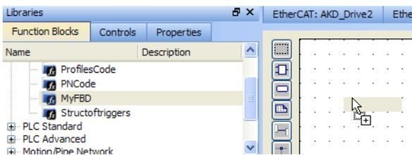
**Figure 4-93:** Create an Instance of UDFB in a Program**NOTE**
