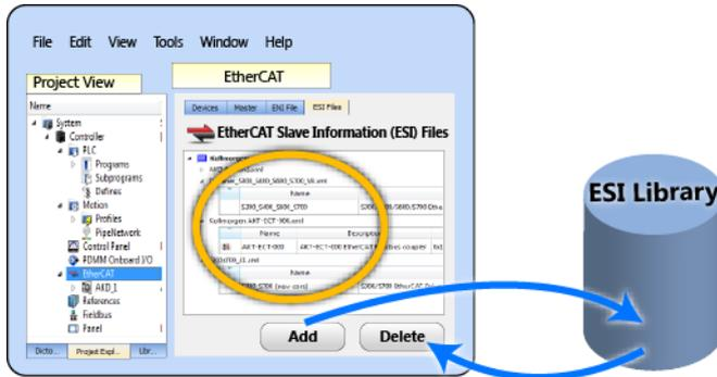
**Figure 4-109: Adding/Deleting** — Adding or deleting an ESI file from the KAS-IDE affects KAS's internal library of ESI files.
