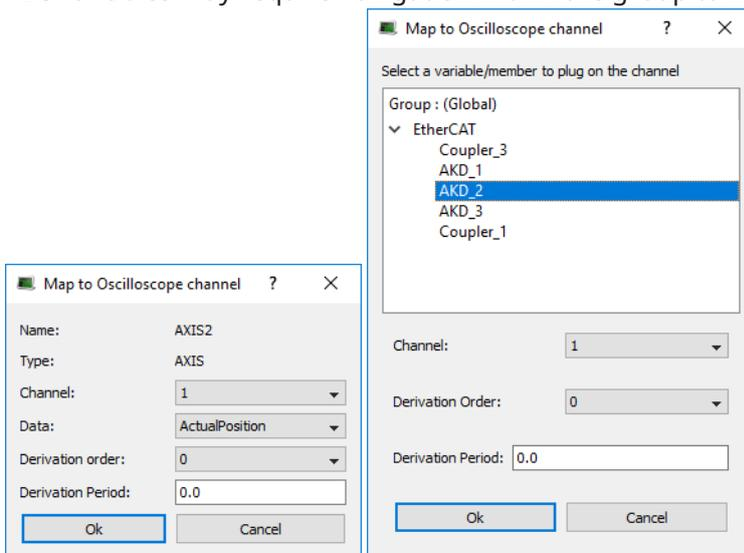
**Figure 5-58:** Associating a Pipe Network (left) and PLCopen (right) variable to a Channel.
