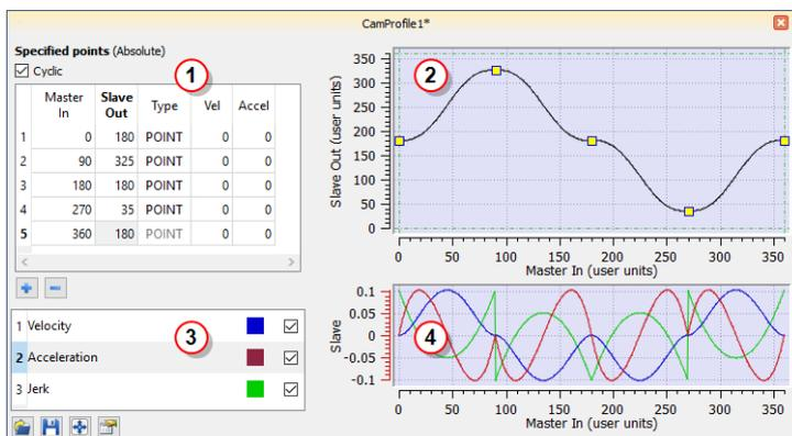
**Figure 5-21:** Cam Profile Editor Main Window
