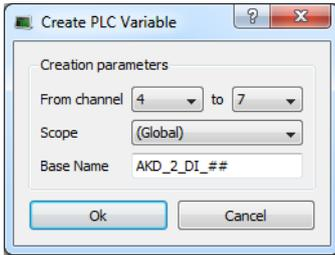
Figure 4-96: Wizard to Create PLC Variable - Parameters
