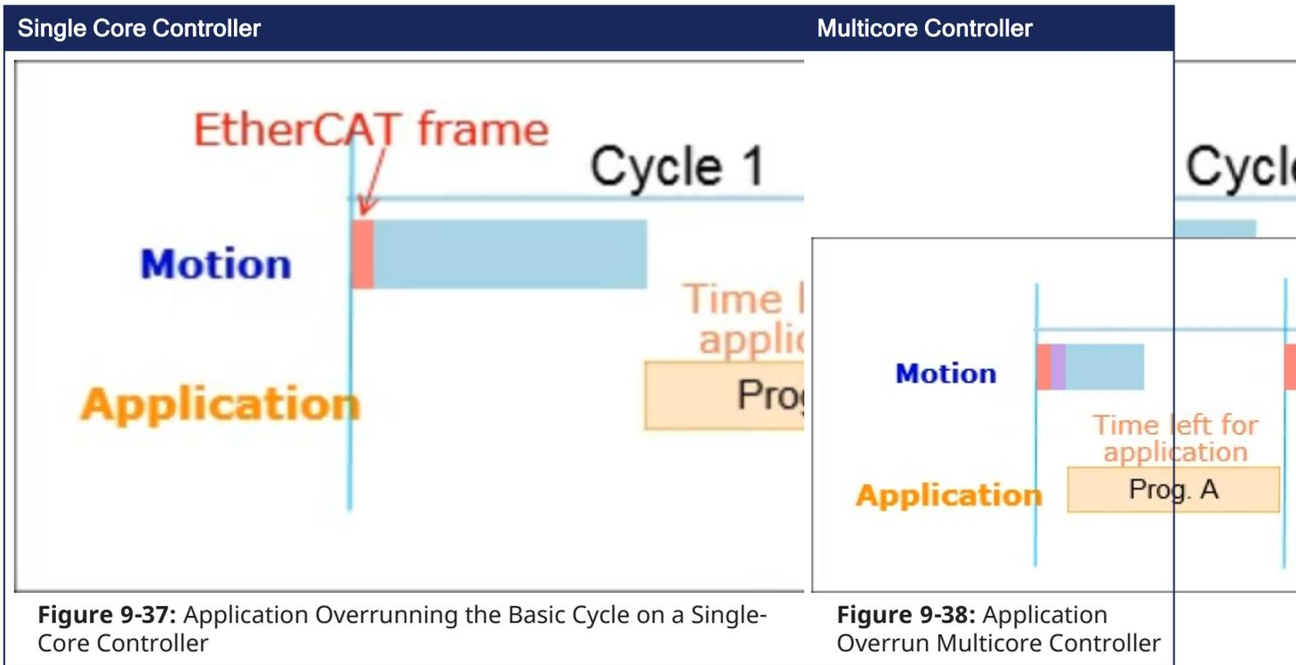
The "Application Overrunning the Basic Cycle on a Single-Core Controller" (→ p. 882) image is an example of an application with two PLC programs (A and B). It takes two cycles to execute all the code in the two programs.
