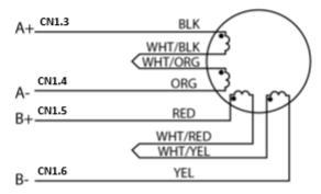
EIGHT LEAD MOTOR CONNECTED IN SERIES
