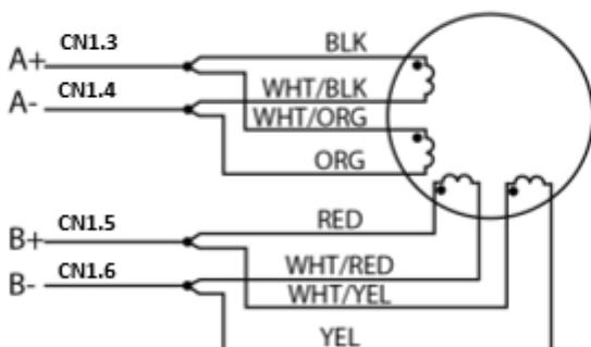
EIGHT LEAD MOTOR CONNECTED IN PARALLEL
