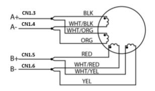
EIGHT LEAD MOTOR CONNECTED IN PARALLEL
