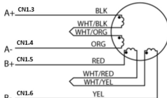
EIGHT LEAD MOTOR CONNECTED IN SERIES
