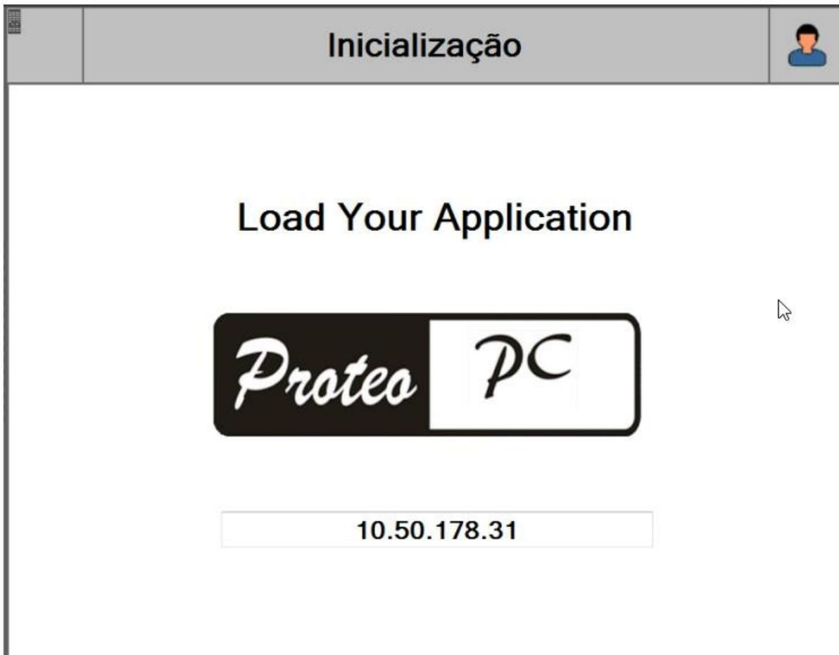
According to the message on the screen, we must load the application on the CNC. There are 3 ways to do this configuration:
